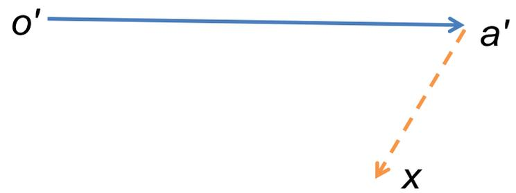
4. From point  $x$ , draw vector  $xb'$  perpendicular to  $AB$  or vector  $a'x$  (because tangential component of  $B$  with respect to  $A$  i.e.  $a_{BA}^t$ , is perpendicular to radial component  $a_{BA}^r$ ) and through  $o'$  draw a line parallel to the path of  $B$  to represent the absolute acceleration of  $B$  i.e.  $a_B$ . The vectors  $xb'$  and  $o'b'$  intersect at  $b'$ . Now the values of  $a_B$  and  $a_{BA}^t$  may be measured, to the scale.
