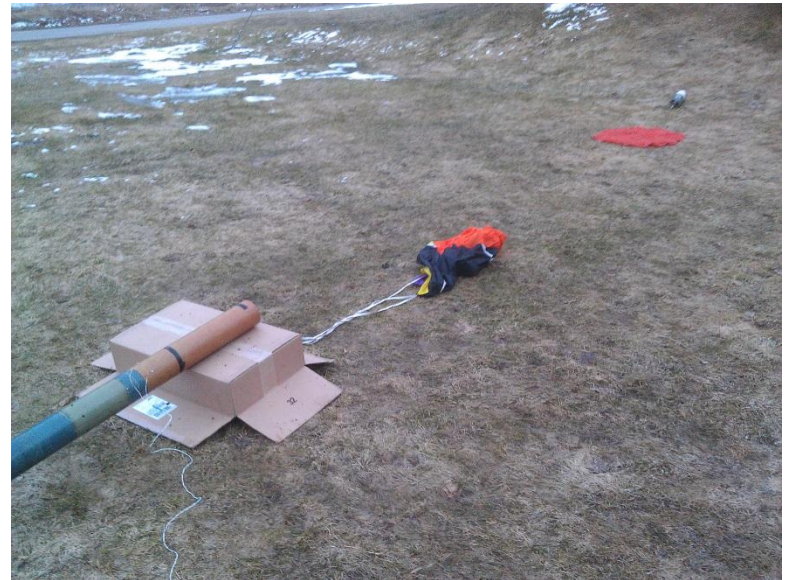
Successful deployment of main parachute and nose cone by main parachute charge.
