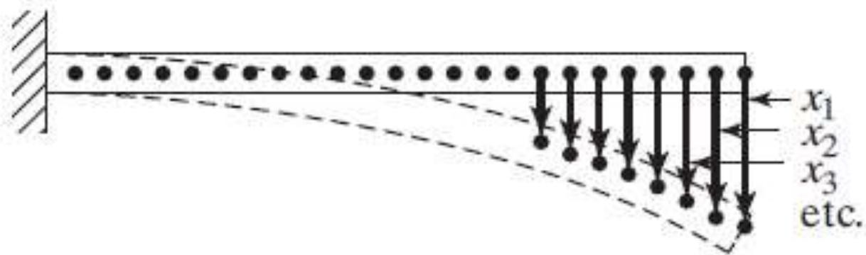
**FIGURE 1.14** A cantilever beam (an infinite-number-of-degrees-of-freedom system).
