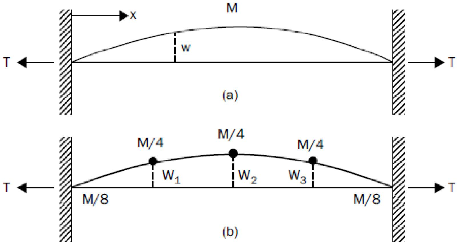
(a) A continuous string of mass  $M$ , displaced transversely;
