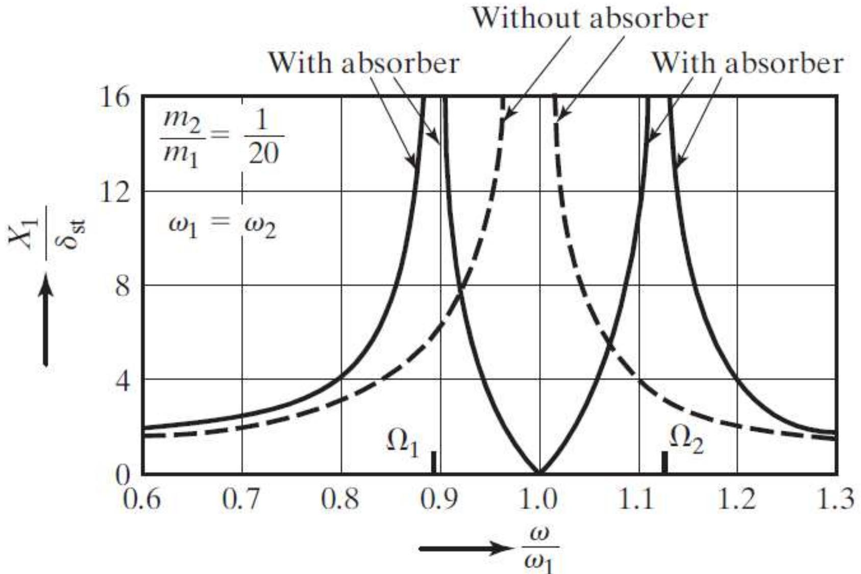
Effect of undamped vibration absorber on the response of machine
