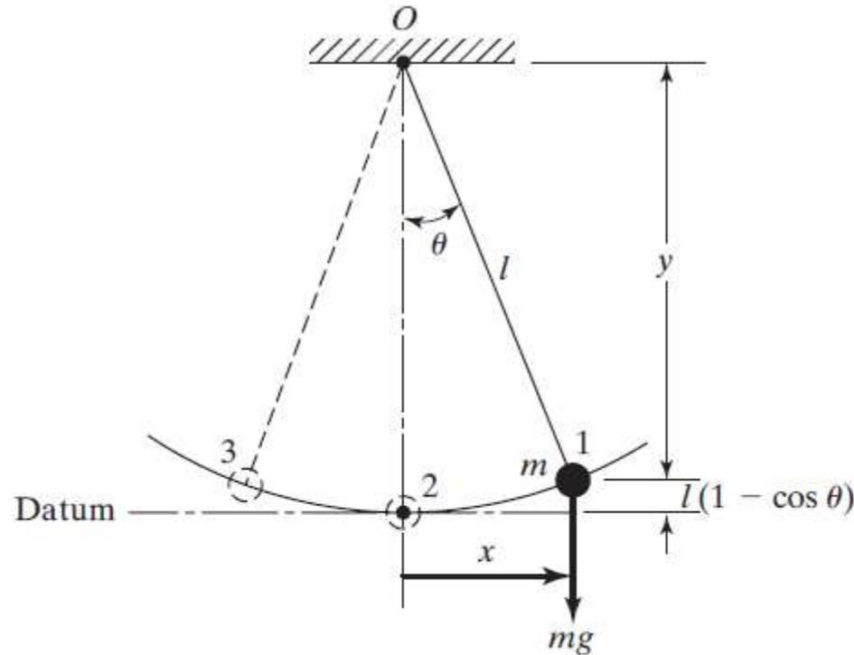
“Period of vibration” is the time that it takes to complete one cycle. It is measured in seconds.
