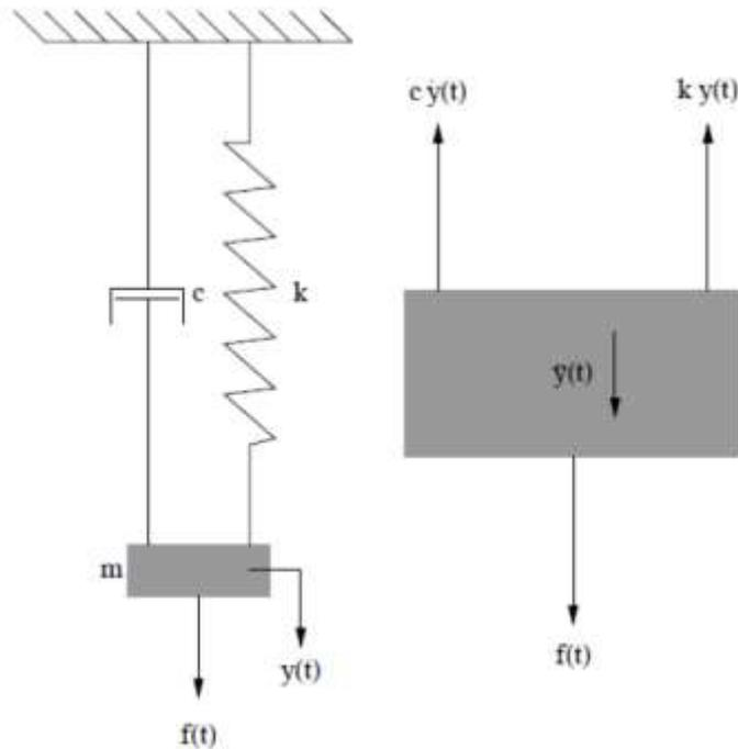
$$y(t) = A_1 e^{p_1 t} + A_2 e^{p_2 t} = e^{-(c/2m)t} \left( A_1 e^{\left(\sqrt{(c/2m)^2 - \omega^2}\right)t} + A_2 e^{-\left(\sqrt{(c/2m)^2 - \omega^2}\right)t} \right)$$
