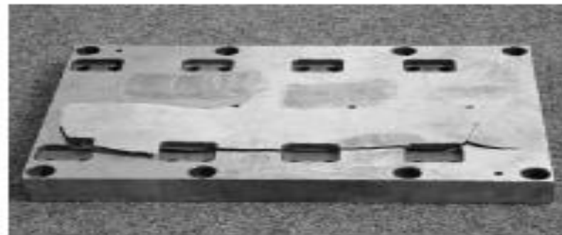
(c) Crack initiation during spark erosion due to high internal stresses, caused by grinding without sufficient cooling (hardened and tempered plate of steel grade 90MnCrV8 (steel number 1.2842).
