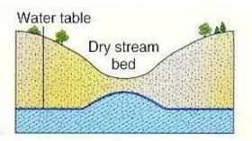
Water table can be close to the land surface beneath a dry stream bed
