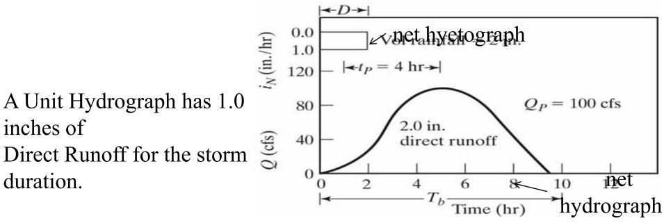
To get a unit hydrograph, UH, first we remove the base flow amount from the hydrograph, as shown, and calculate the net rainfall by removing the infiltration and retention storage from the hyetograph. Then scale the new hydrograph units to yield a unit hydrograph for, say, 1 inch for one hour, or 1/2 in/hr for 2 hours, or 1/3 in/hr for 3 hr, etc.
