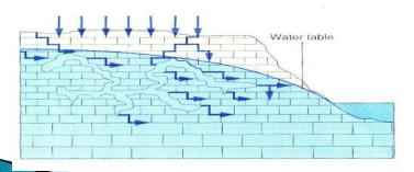
Water moves along fractures and bedding planes in limestone, dissolving a dimestone to form caves below the water table
