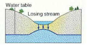
Stream losing water through stream bed to saturated zone
