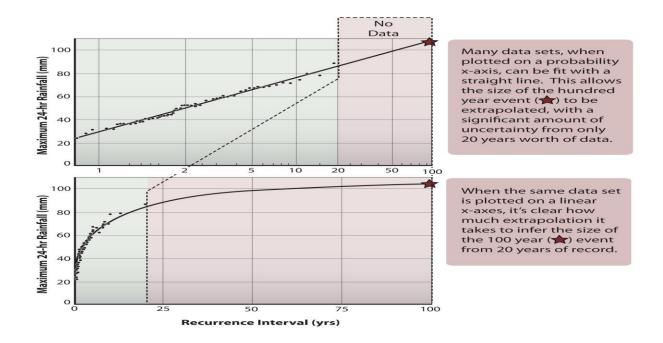
Figure 4.2 - Precipitation Recurrence Interval with Extrapolation (chapter 4 - Hydrology)
