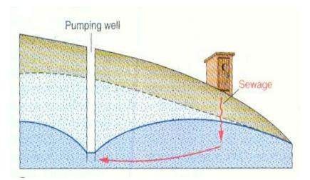
Water-table slope is reversed by pumping, changing direction of the ground-water flow, and polluting the well
