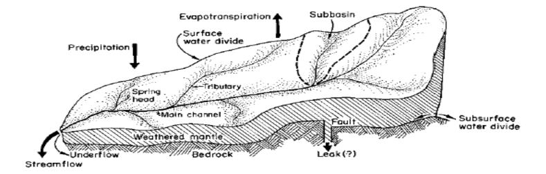
Fig 2-3. Diagram showing terms essential to describe the drainage basin and its water balance. Underflow is unmeasured streamflow in sands, gravels and rocks beneath the channel bed.
