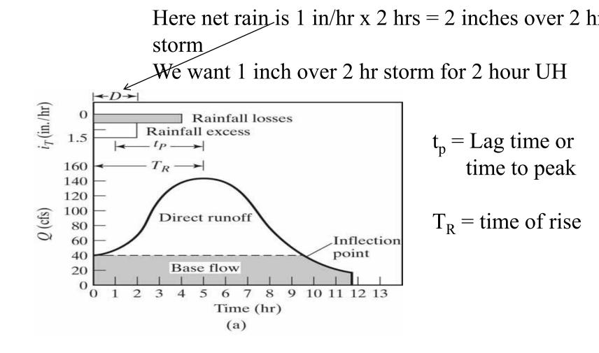
A typical Storm gross hyetograph and gross hydrograph. The gross hydrograph can be converted to a unit hydrograph (1 inch over 1 hour, .5 inches over 2 hours, .33333 inches over 3 hours, etc.) by subtracting the base flow (gives a net hydrograph), calculating the total Direct Runoff flow from the net hyetograph, then scaling the hydrograph ordinates by the same multiplier to give the total flow of 1 inch over the storm duration.
