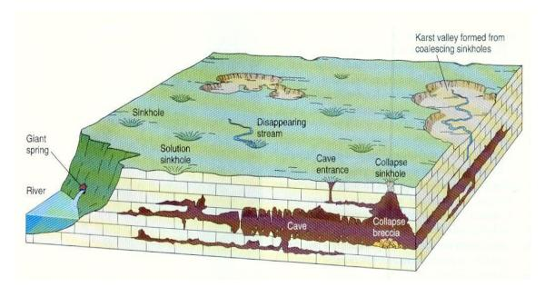
Karst top-graphy is marked by underground caves and numerous surface sinkholes. A major river may cross the region, commall surface streams generally disappear down sinkholes
