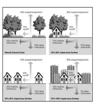
Figure 1.2: Relationship Between Impervious Cover and Surface Runoff Source: Federal Interagency SRWG, 2000
