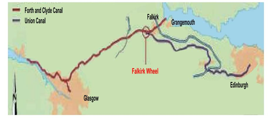
At the beginning there were two canals: Canal Forth and Clyde was built in 1777 Canal Union between Falkirk and Edinburgh was finished in 1822 Because of geographical difficulties, which created a difference of 79ft.in elevation, the two canals were connected by 11 locks.
