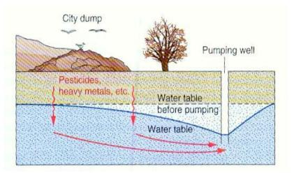
Water table steepens near a dump, increasing the velocity of ground-water flow and drawing pollutants into a well
