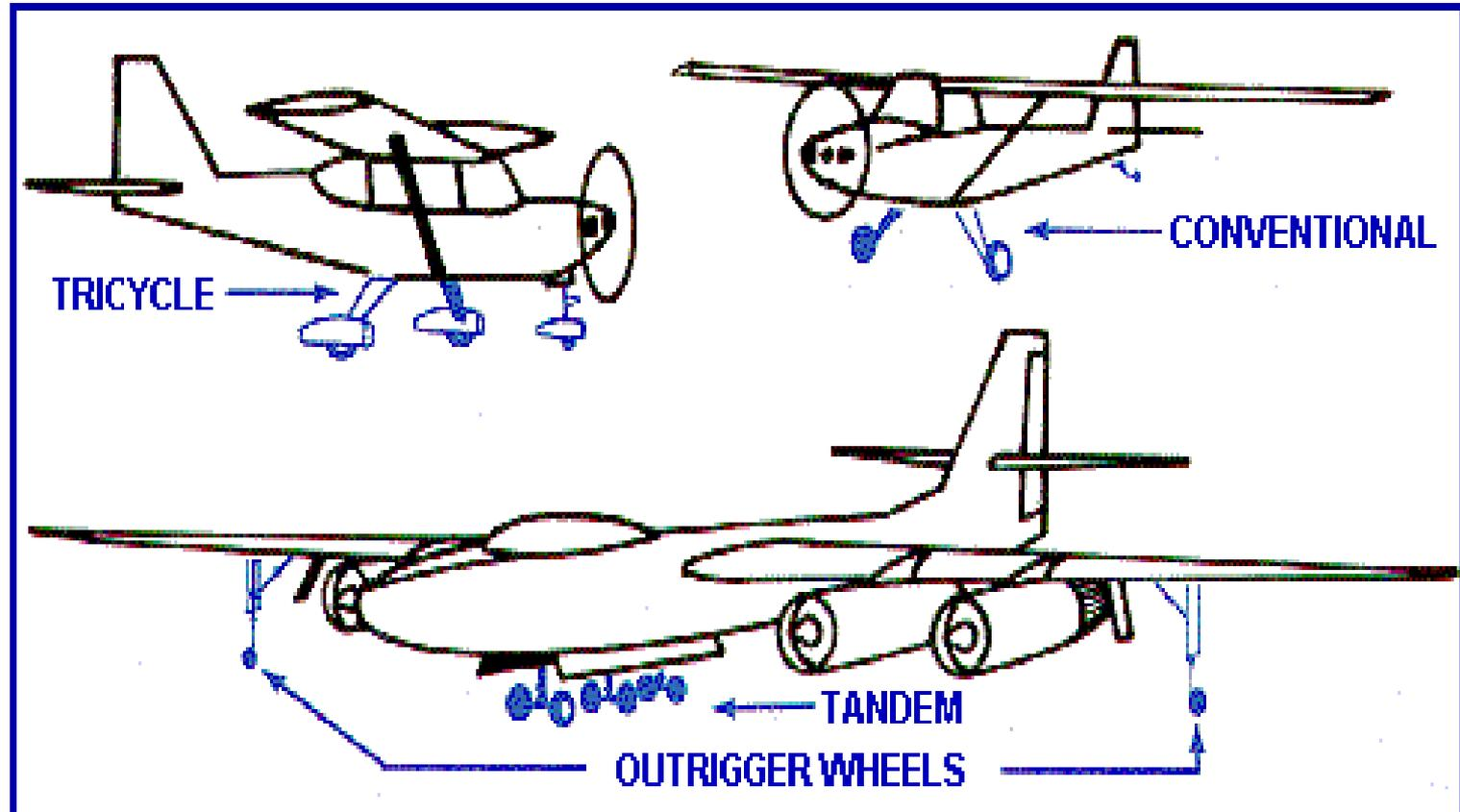
Figure 1-8 Three basic types of landing gear arrangements
