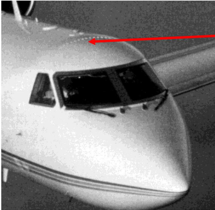
Shock wave causes flow separation in this region. Vortex generators fix problem. However, shock wave remains causing drag and considerable.
