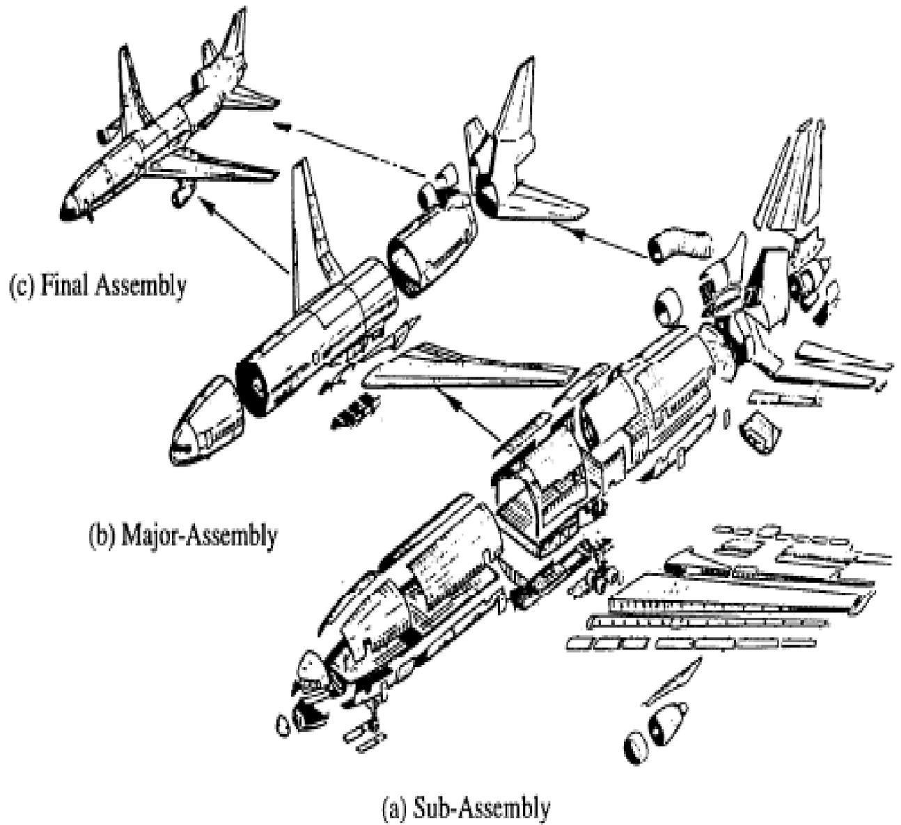
*Fig. 1.4.2 Lockheed L-1011's Sub-assemblies and Final Assembly*
