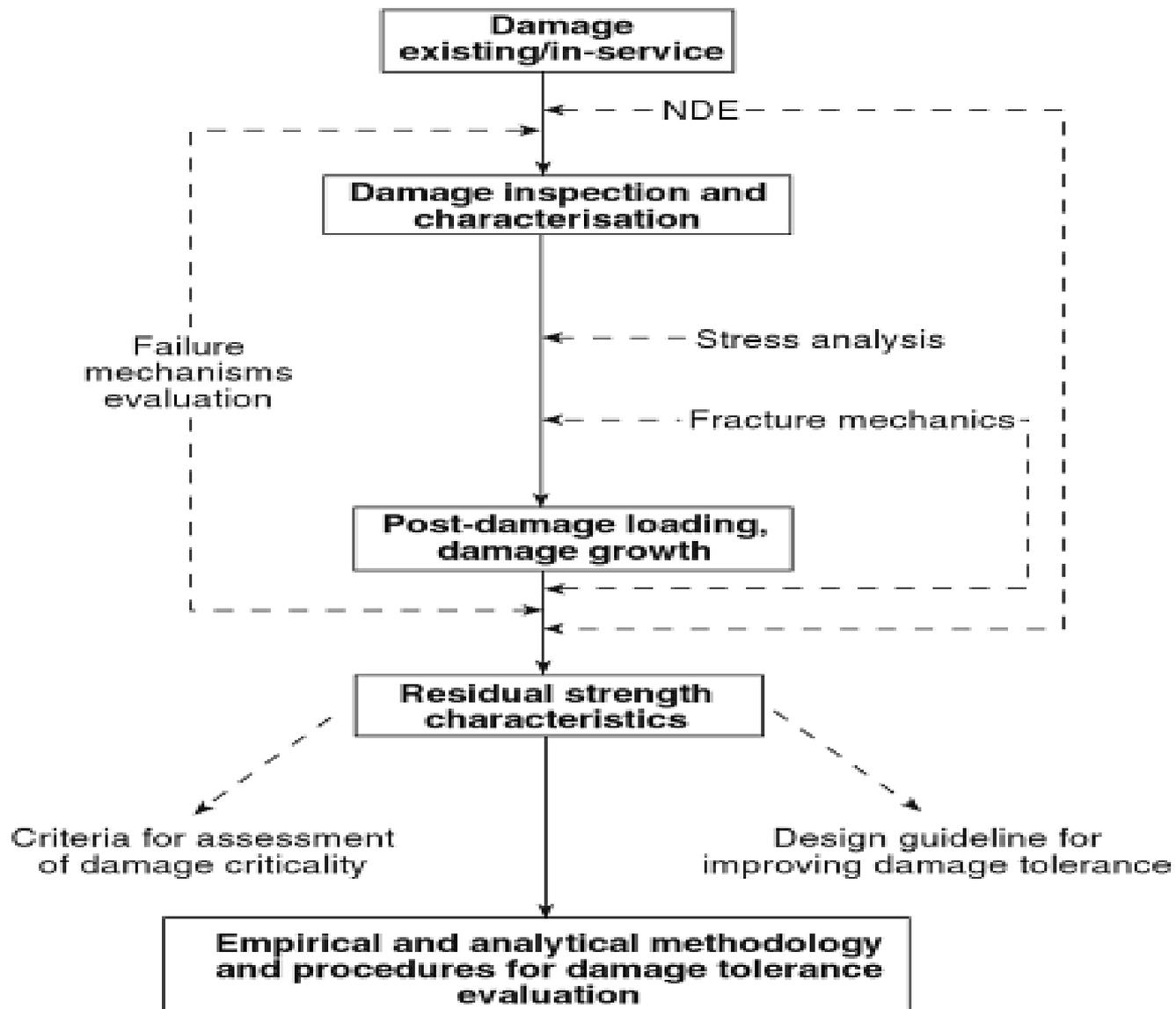
Damage tolerance concepts.
