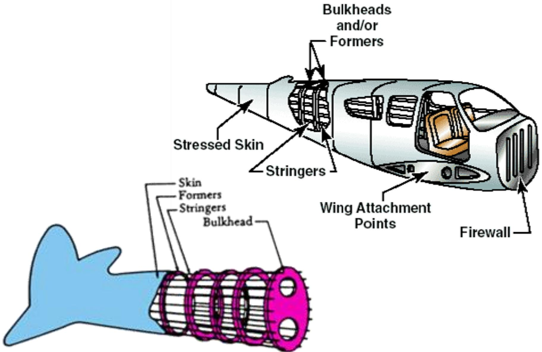
Semi-monocoque Structure of an airplane
