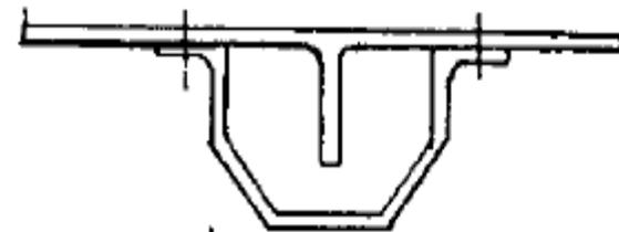
*(d) Blade section with reinforcement*
