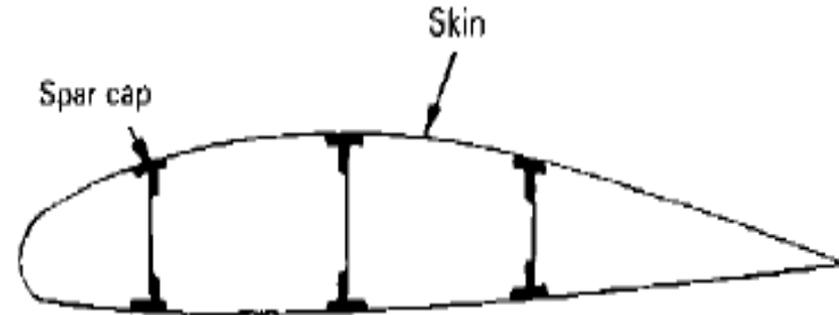
**Three spar wing - all bending materials concentrated at the spar caps**
