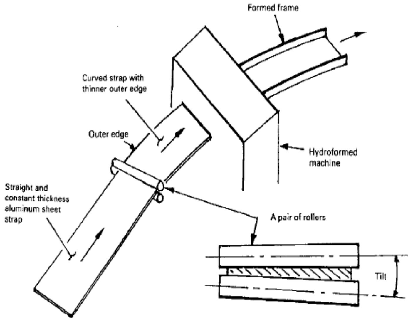
*A common process of forming fuselage frame.*
