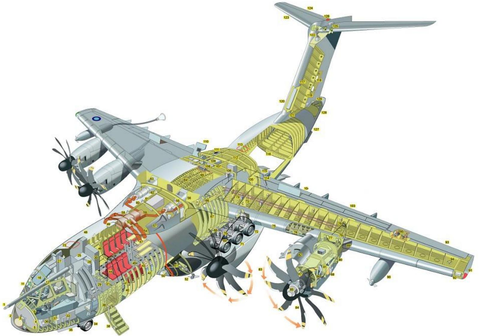
Semi-monocoque Structure of an airplane
