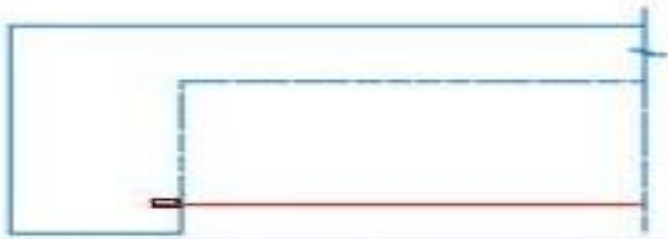
Step#4: Installing dowels for the main steel.
