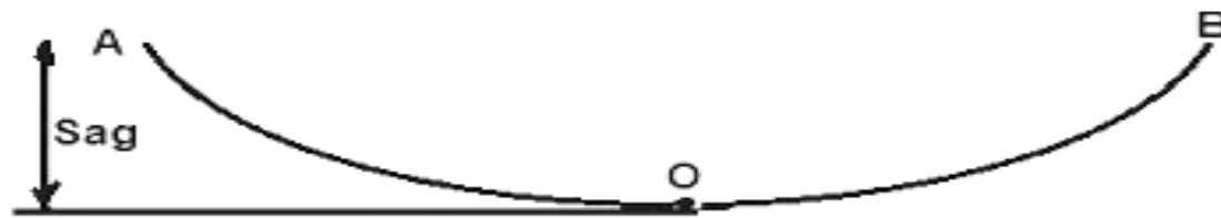
Fig.1: Sag in a transmission line
