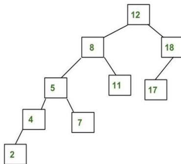
The above tree is not AVL because differences between heights of left and right subtrees for 8 and 18 is greater than 1.
