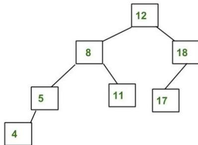
The above tree is AVL because differences between heights of left and right subtrees for every node is less than or equal to 1.
