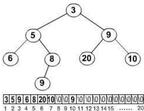
The figure shows how a binary tree is represented as an array. The root 3 is the 0<sup>th</sup> element while its leftchild 5 is the 1<sup>st</sup> element of the array. Node 6 does not have any child so its children i.e. 7<sup>th</sup> and 8<sup>th</sup> element of the array are shown as a Null value.
