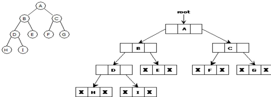
Binary trees can be represented by links where each node contains the address of the left child and the right child. If any node has its left or right child empty then it will have in its respective link field, a null value. A leaf node has null value in both of its links.
