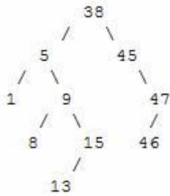
could result in losing sub trees that are rooted at 1 and 9. Hence we need to be careful about deleting nodes from a tree. The best way to deal with deletion seems to be considering special cases. What if the node to delete is a leaf node? What if the node is a node with just one child? What if the node is an internal node (with two children). The latter case is the hardest to resolve. But we will find a way to handle this situation as well.
