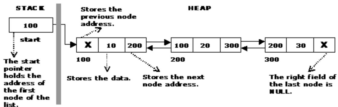
The beginning of the double linked list is stored in a "start" pointer which points to the first node. The first node's left link and last node's right link is set to NULL.
