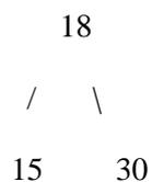
A Perfect Binary Tree of height  $h$  (where height is number of nodes on path from root to leaf) has  $2^h - 1$  node.
