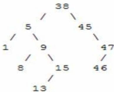
Then we find the largest node in the left sub tree (15) or smallest node in the right sub tree (45) and replace the root with that node and then delete that node. The following set of images demonstrates this process.
