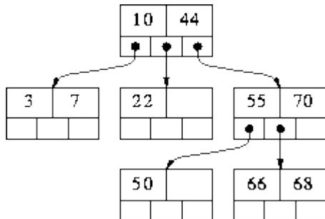
In our examples it will be convenient to illustrate M-way trees using a small value of M. But bear in mind that, in practice, M is usually very large. Each node corresponds to a physical block on disk, and M represents the maximum number of data items that can be stored in a single block. M is maximized in order to speedup processing: to move from one node to another involves reading a block from disk - a very slow operation compared to moving around a data structure stored in memory.
