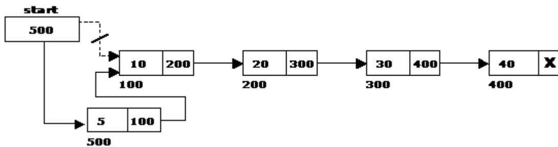
**Inserting a node at the end:**
