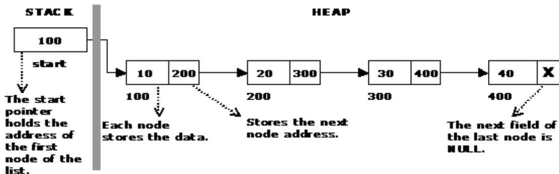
The beginning of the linked list is stored in a "start" pointer which points to the first node. The first node contains a pointer to the second node. The second node contains a pointer to the third node, ... and so on. The last node in the list has its next field set to NULL to mark the end of the list. Code can access any node in the list by starting at the **start** and following the next pointers.
