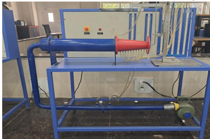
Fig. 23: Nozzle performance test rig
