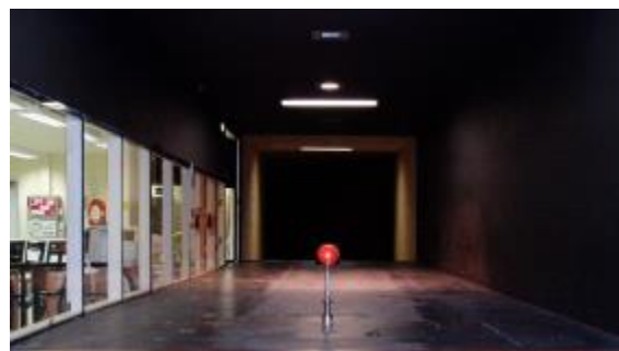
Fig. 26: Experimental setup to study cricket ball [Alam et. al, 2010]
