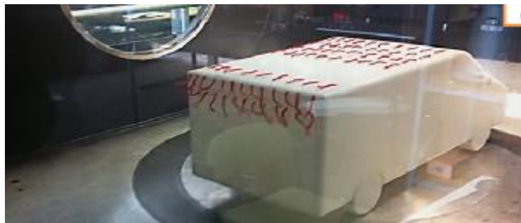
Fig. 8: Tuft flow visualization over the model car
