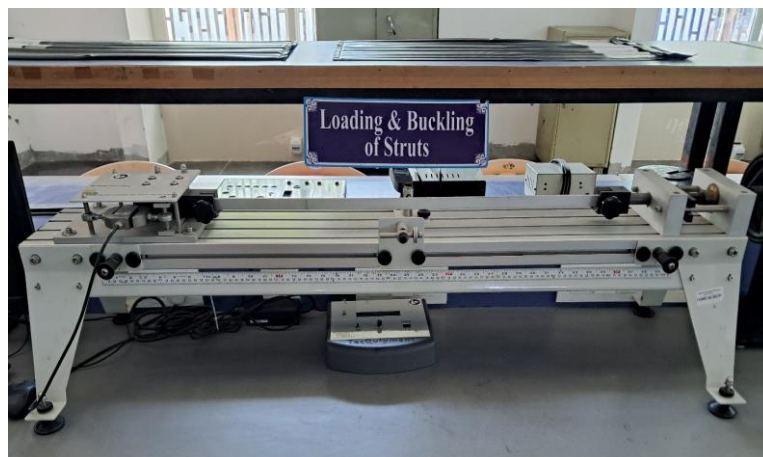
Fig. 3.1: Loading and buckling of struts equipment
