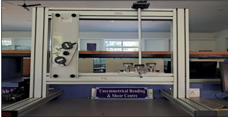
Fig. 6.1: Equipment for determination of shear centre of an open section beam
