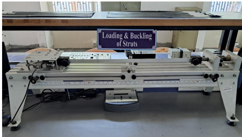
Fig. 4.1: Loading and buckling of struts equipment for compression test
