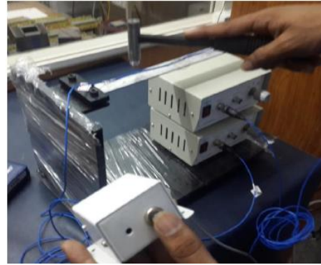
Fig 13.3: Showing impact loading with trigger
