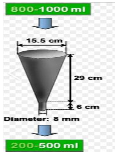
Fig. 7.1. Marsh Cone test
