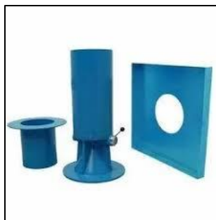
Fig 5.1: Sand replacement test equipment
