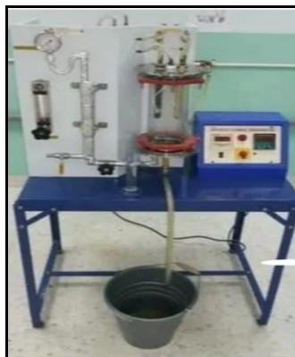
Figure 14.1 Film and Drop Wise Condensation
