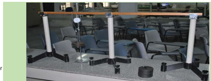
fig.12.2: Setup of Continuous beam deflection
