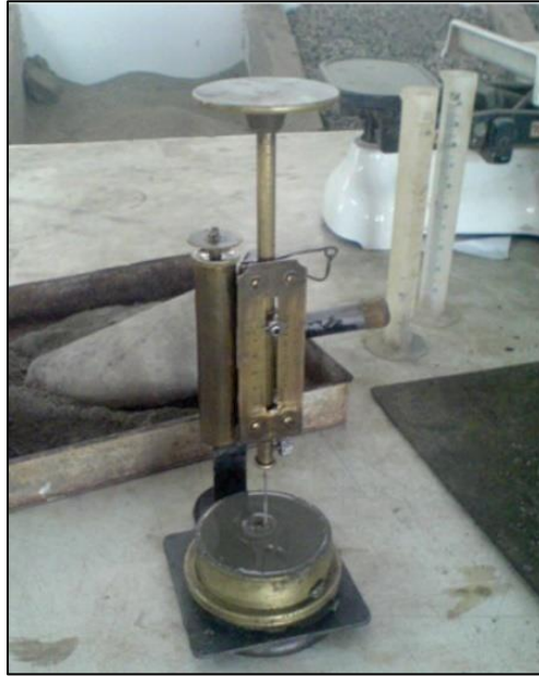
Fig:11 Vicat Apparatus for setting time of cement.
