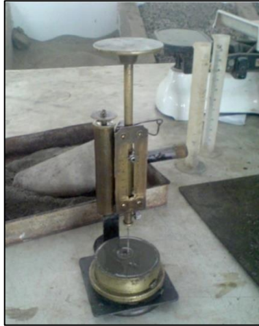
Fig:10 Vicat apparatus for Normal Consistency of cement.
