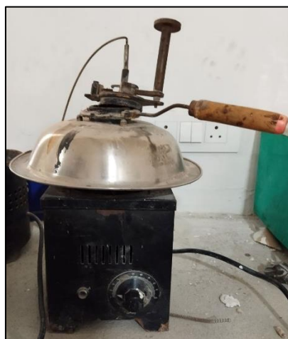
Fig: 9 Flash and Fire Point, IS Standards used: IS: 1209-1978.
