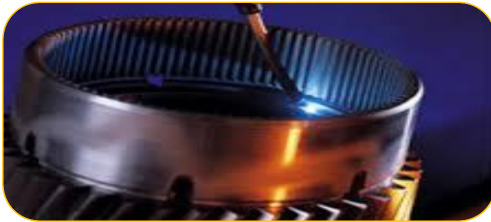
Laser surface treatment to change the micro structure of metals through controlled heating and cooling.
