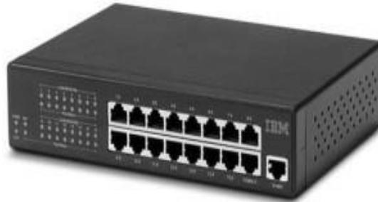
Switch is also one of the connecting device but the difference between hub and switch is working that hub works by sending the data to all the ports on the device whereas a switch transfers it only to that port which is connected to the destination device. Switches operate in full-duplex mode where devices can send and receive data from the switch.
