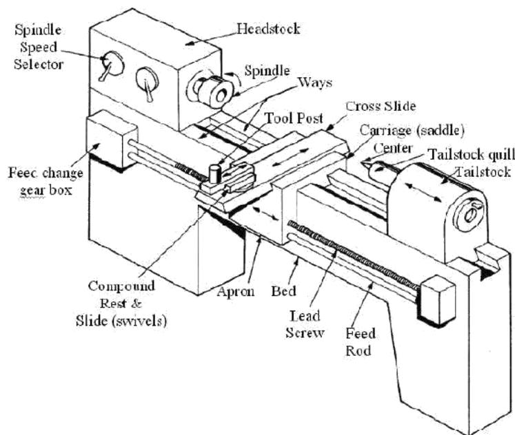
A lathe is a machine tool which rotates the workpiece on its axis to perform various operations such as cutting, sanding, knurling, drilling, or deformation with tools that are applied to the workpiece to create an object which has symmetry about an axis of rotation.
