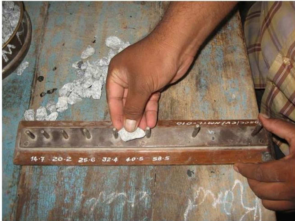
Elongation Index Test in Progress
