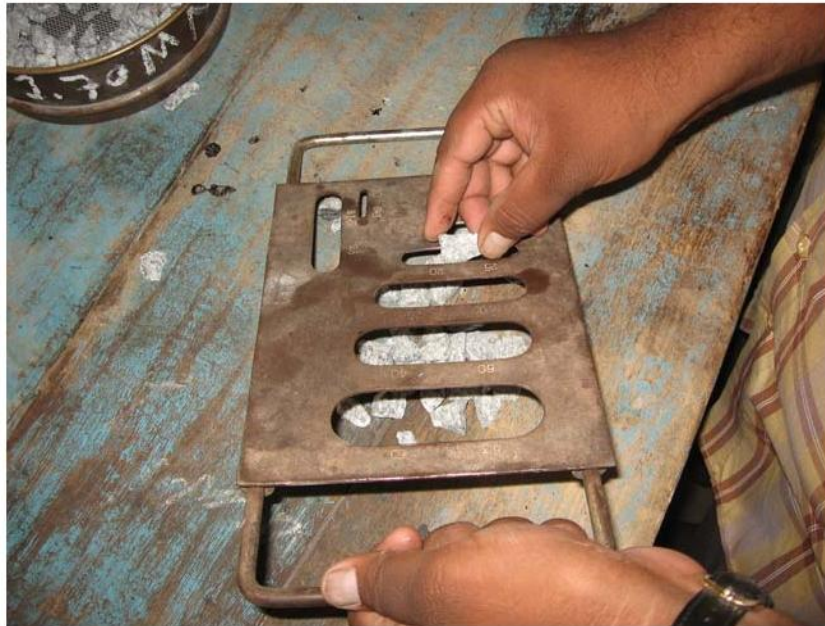
Flakiness Index Test in Progress
