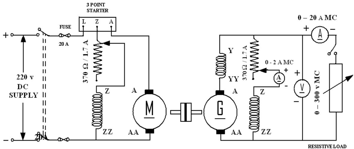
**Fig - 4.1 DC Shunt Motor - Compound Generator Set**
