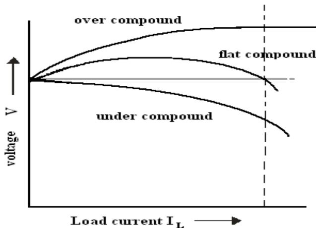
**Fig – 4.2 Load Characteristics of DC Compound Generator**
