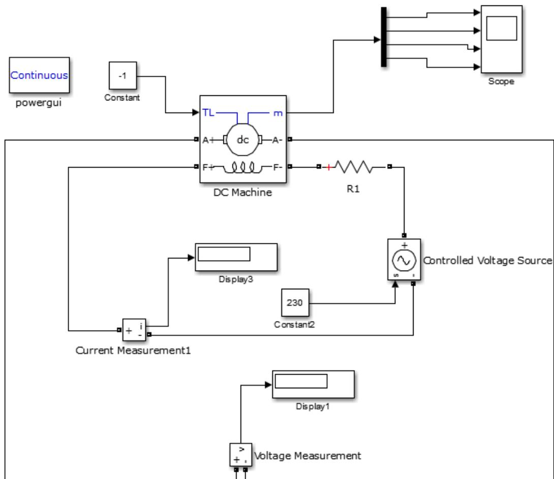
Fig - 12.1 DC Shunt Motor - Shunt Generator Set
