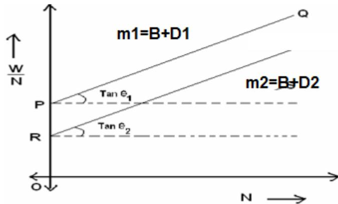
Fig – 11.2 Separation of Losses
