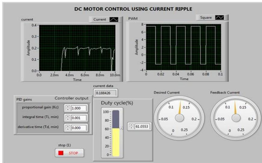
**Fig - 14.2 Closed loop controlling of DC motor**
