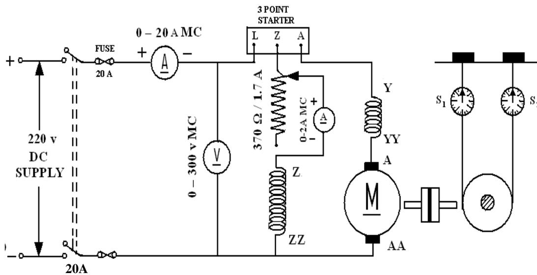
**Fig – 8.1 DC Compound Motor with Brake Drum**
