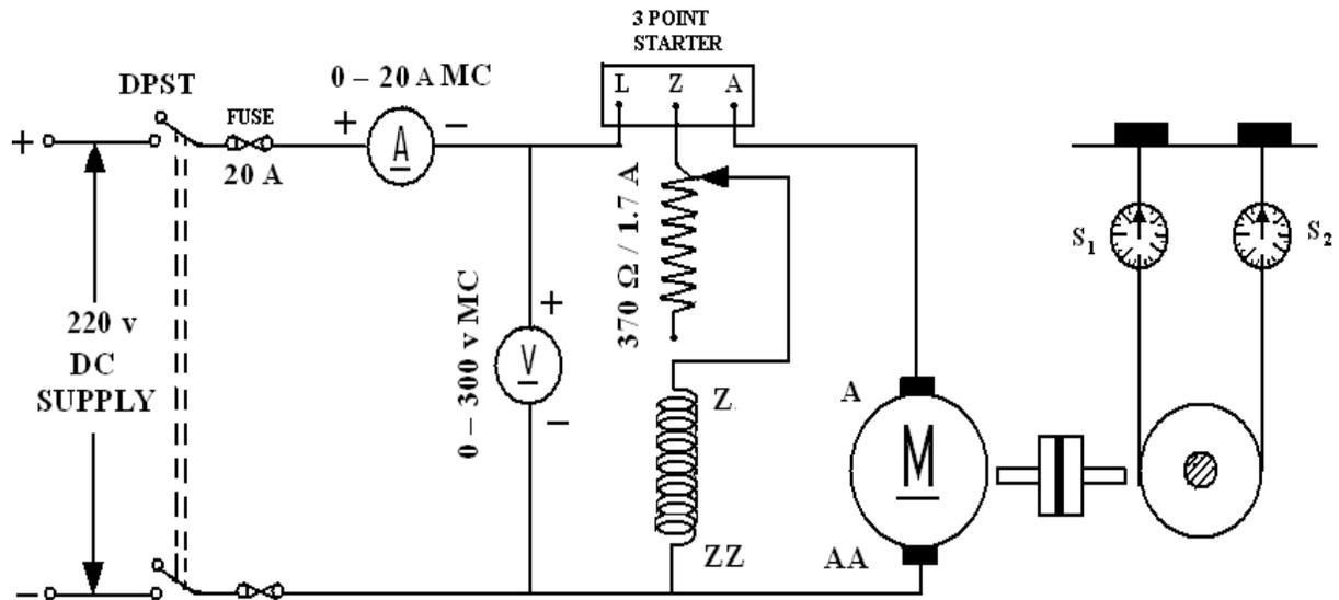
**Fig – 9.1 DC Shunt Motor with Brake Drum**
