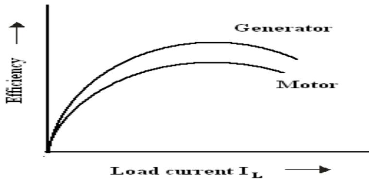
**Fig – 7.2 Load Characteristics of DC Shunt Motor and Generator**
