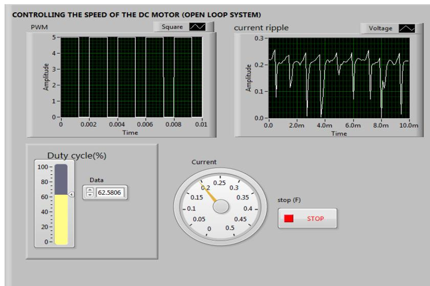
**Fig - 14.1 - Front Panel of Open Loop Control of DC Motor**
