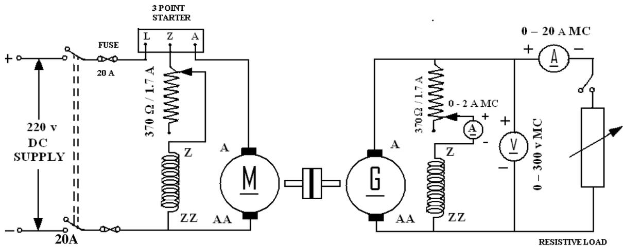
**Fig - 2.1 DC Shunt Motor - Shunt Generator Set**
