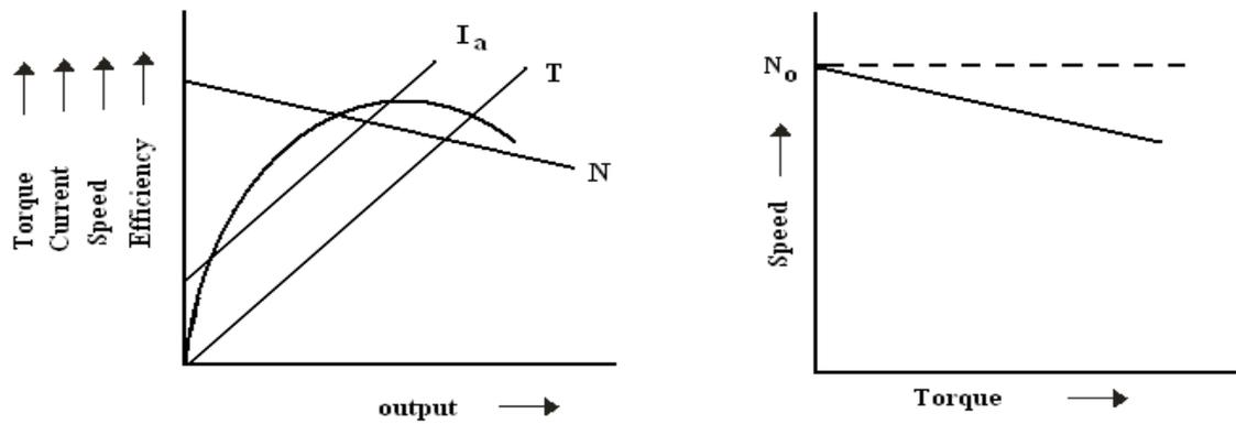
**Fig – 9.2 Performance Characteristics of DC Shunt Motor**
