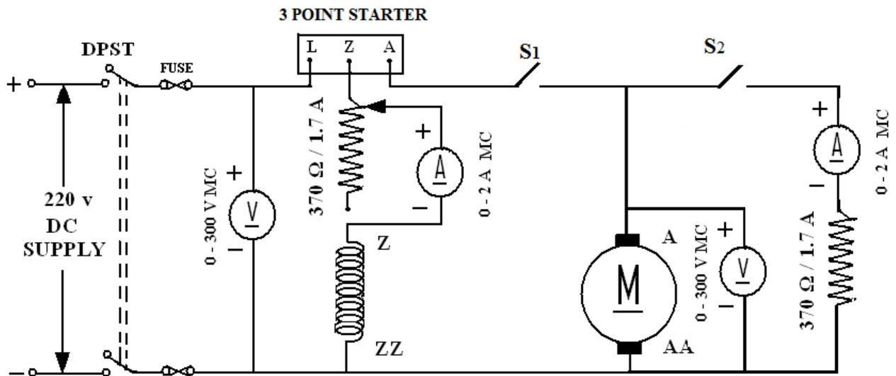
**Fig – 10.1 DC Shunt Motor**
