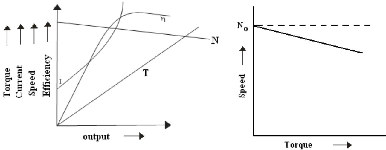
**Fig – 8.2 Performance Characteristics of Compound Motor**
