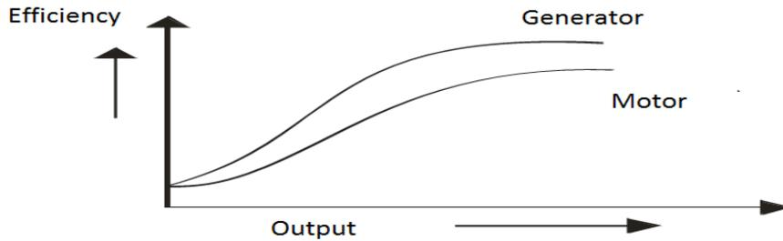
**Fig – 5.2 Efficiency of Identical DC shunt machines**
