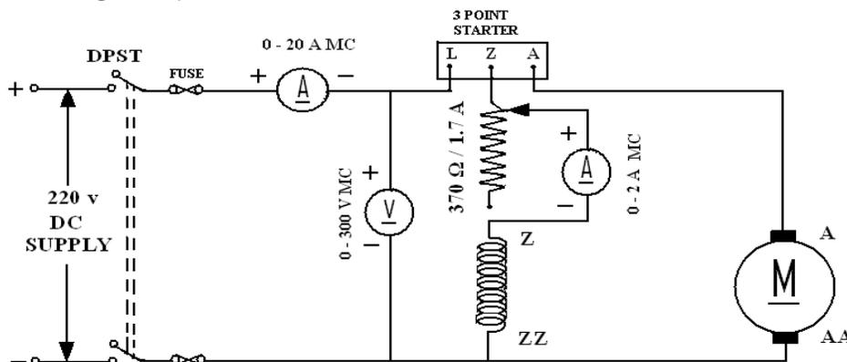
**Fig – 7.1 DC Shunt Motor**
