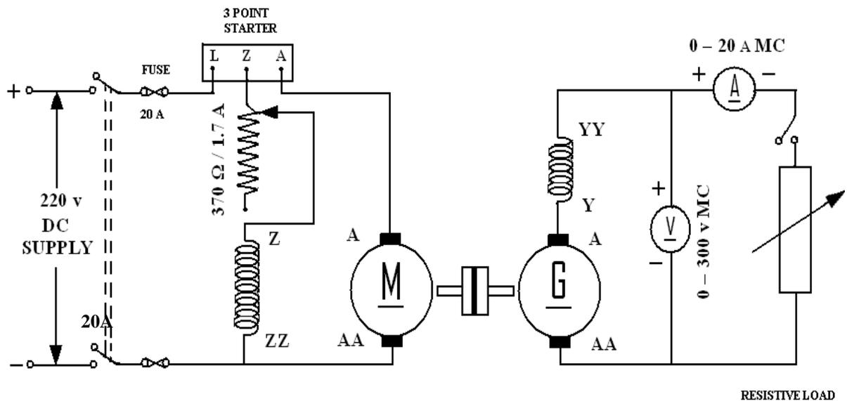
**Fig - 3.1 DC Shunt Motor - Series Generator Set**
