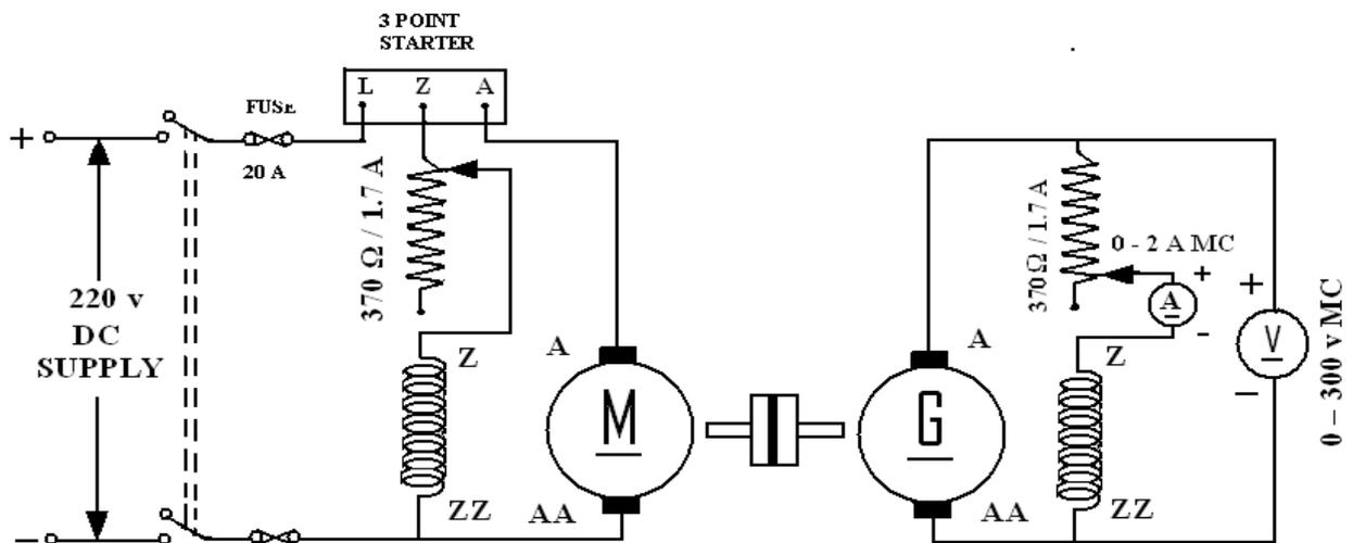
Fig - 1.1 DC Shunt Motor - Shunt Generator Set
