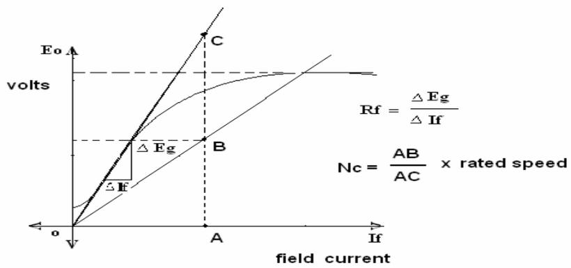
**Fig - 12.2 Magnetization Characteristics Curve**
