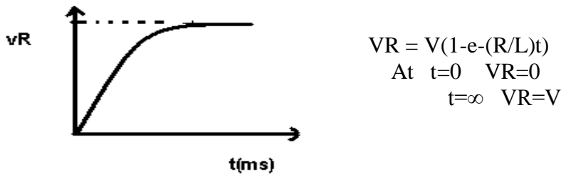
Fig – 1.7 Output Voltage Wave across Resistor
