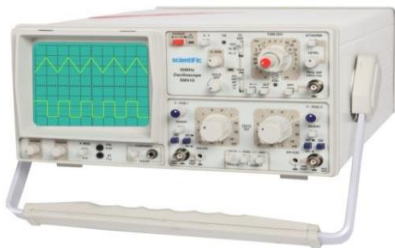
Fig 1. Cathode Ray tube Oscilloscope Fig 2. Out Line Diagram of CRO
