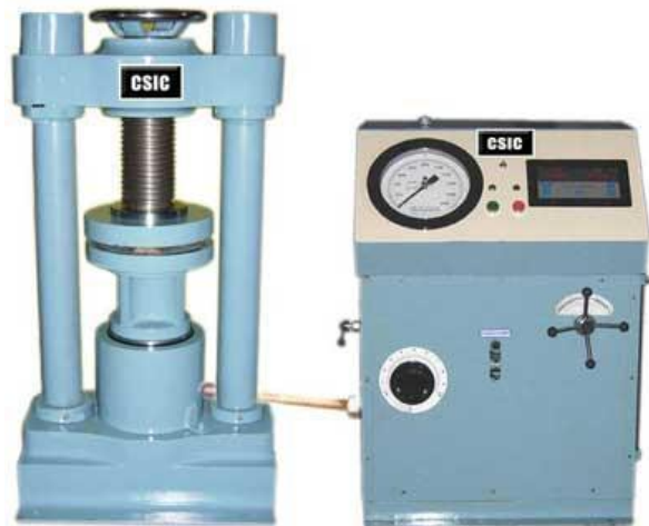
Fig: Compressive Strength Test on Concrete
