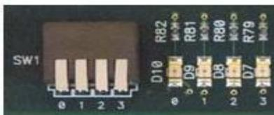
The DSK implements the logic necessary to tie board components together in a programmable logic device called a CPLD. In addition to random glue logic, the CPLD implements a set of 4 software programmable registers that can be used to access the on-board LEDs and DIP
