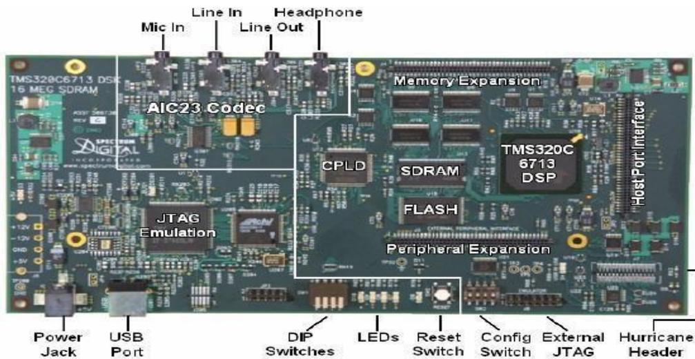
The DSK has 4 light emitting diodes (LEDs) and 4 DIP switches that allow users to interact with programs through simple LED displays and user input on the switches. Many of the included examples make use of these user interfaces Options.
