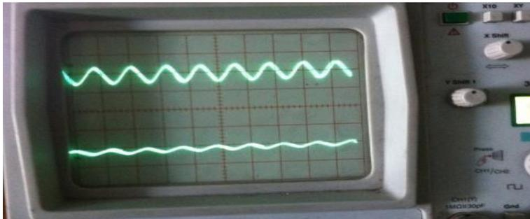
d) function generator (input signal frequency at 1.1kHz)
