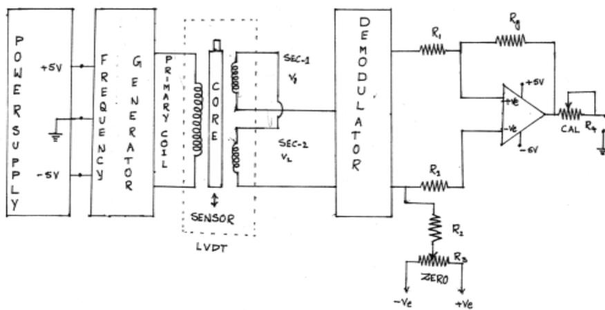
**Fig – 4.1 Circuit Diagram of LVDT and Capacitance Pickup – Characteristics and Calibration**
