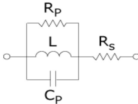
**Figure - 14.3 A Model of Different Parasitic Elements in a Real-World Component That Can Impact the Inductor**
