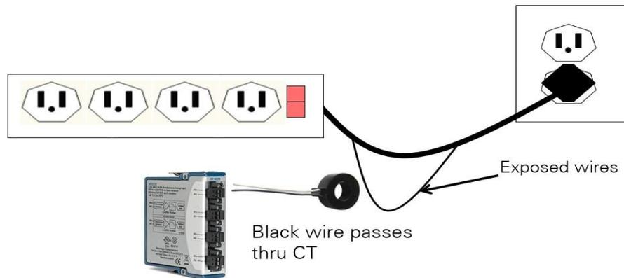
**Figure – 12.4 For module measurement using a CT, the load wire (black in the US), is passed through the opening of the CT either via a split core CT or cutting/re-splicing the wire. The leads from the CT are then connected to the AI+ and AI- of the measurement module. The module will measure all current on the line that is routed through the CT opening. Scaling is done in software to convert from the Voltage/Amp output from the sensor to the full scale Amperage on the circuit.**
