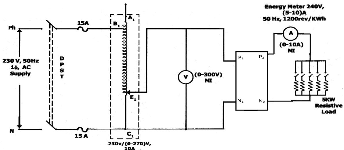
Fig (a) – 6.1 Calibrations and Testing of Single Phase Energy Meter
