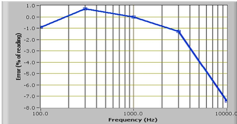
**Fig - 14.5 A 5 mH Air-Core Inductor Measured over Different Frequencies**
