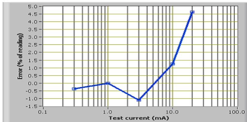
**Fig - 14.6 A 100 uH Ferrite-Core Inductor Tested at Different Test Signal Levels**
