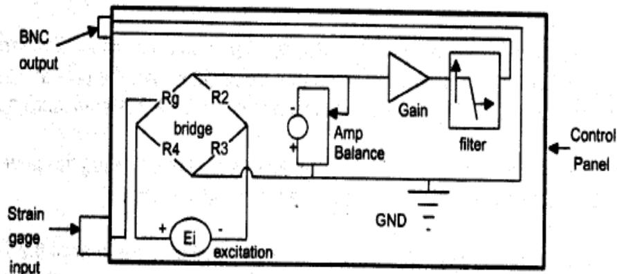
**Fig – 3.1 Circuit Diagram of Resistance Strain Gauge Strain Measurements and Calibration**
