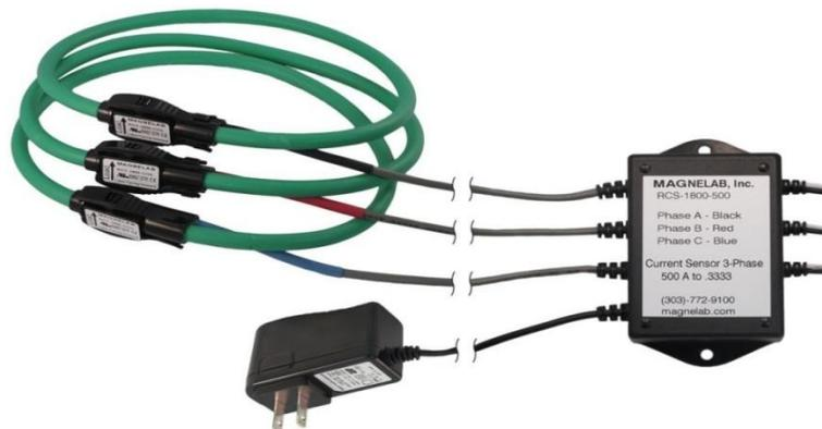
**Figure – 12.7 Rogowski coils require external power, integration circuitry (located in the black mountable box in the image above), and are more expensive than typical solid/split core CTs, but offer fast phase response and are good for retrofit installations and large bus bar measurements due to their large flexible opening. (Image courtesy of Magnelab)**
