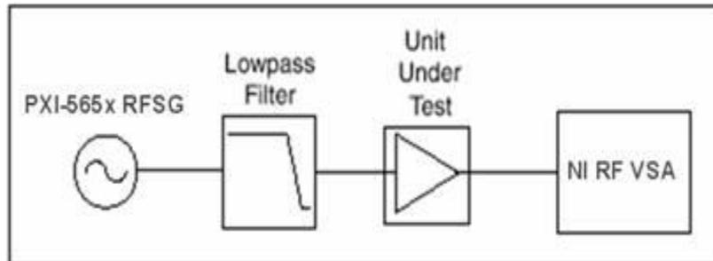
**Fig – 10.2 Typical Harmonic Distortion Measurement Setup**
