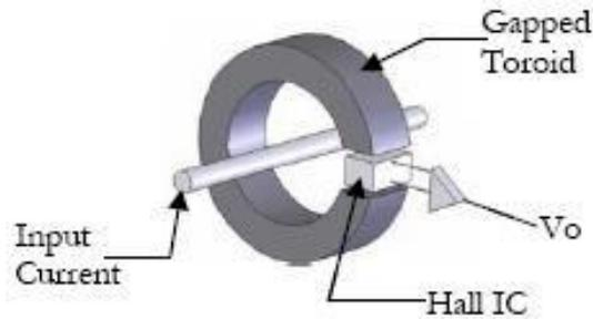
**Figure – 12.8 Hall Effect sensors have a sensing circuit perpendicular to the magnetic field and requires power. Hall Effect sensors are not subject to saturation limits like a CT and can measure DC currents, but are more costly.**
