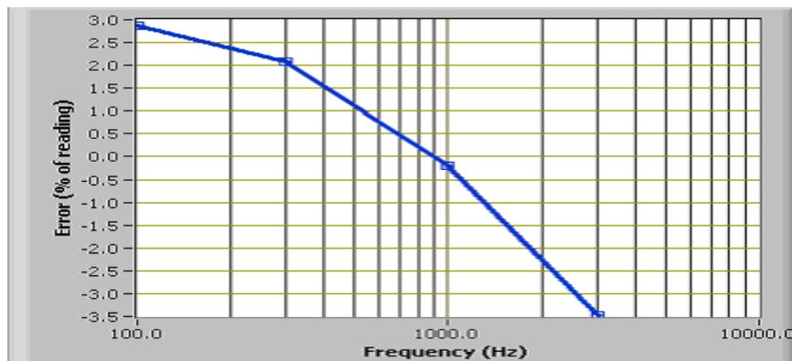
**Figure 14.2 A 2.2  $\mu\text{F}$ , 100 V Aluminum Electrolytic Capacitor Measured at Different Frequencies**
