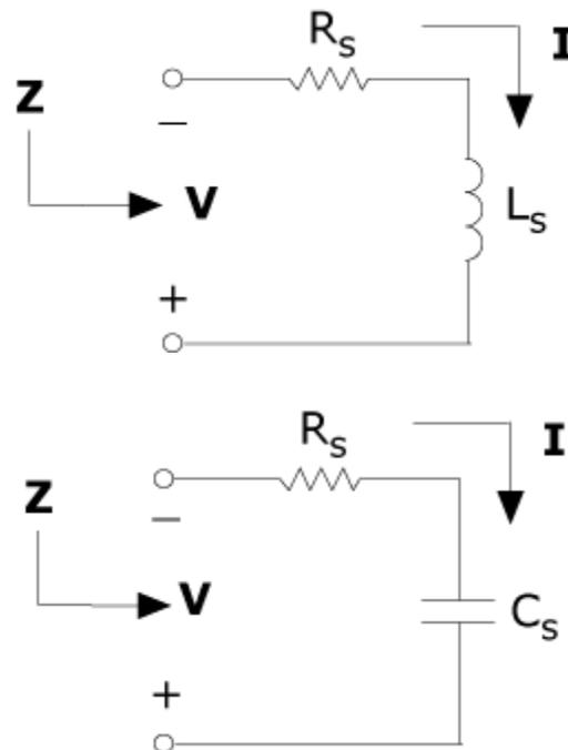
**Fig - 14. 2 You can easily model loads either as a series or parallel combination of a resistive and a reactive load using the formulas above.**
