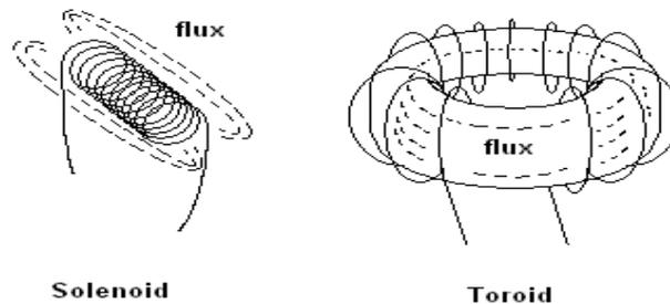
**Figure14.4 Types of Inductor Flux**
