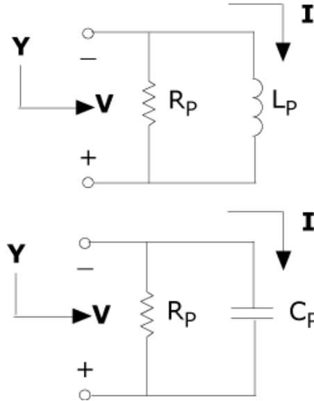
**Fig - 14. 3 It is mathematically easier to manipulate parallel loads as admittances and series loads as impedances.**
