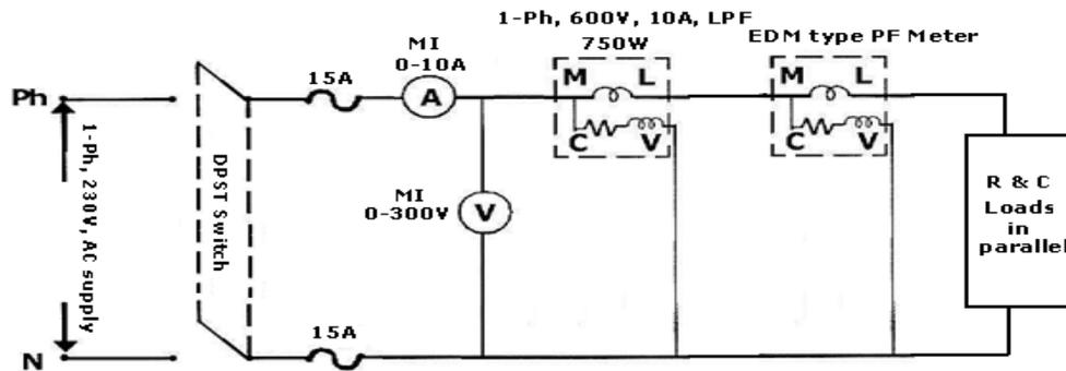
Fig (b) – 6.1 Calibration of Dynamo Meter Type Power Factor Meter
