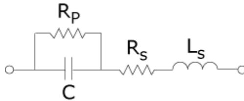
**Figure 14.1 A Model of Different Parasitic Elements in a Real-World Component That Can Impact the Capacitor**
