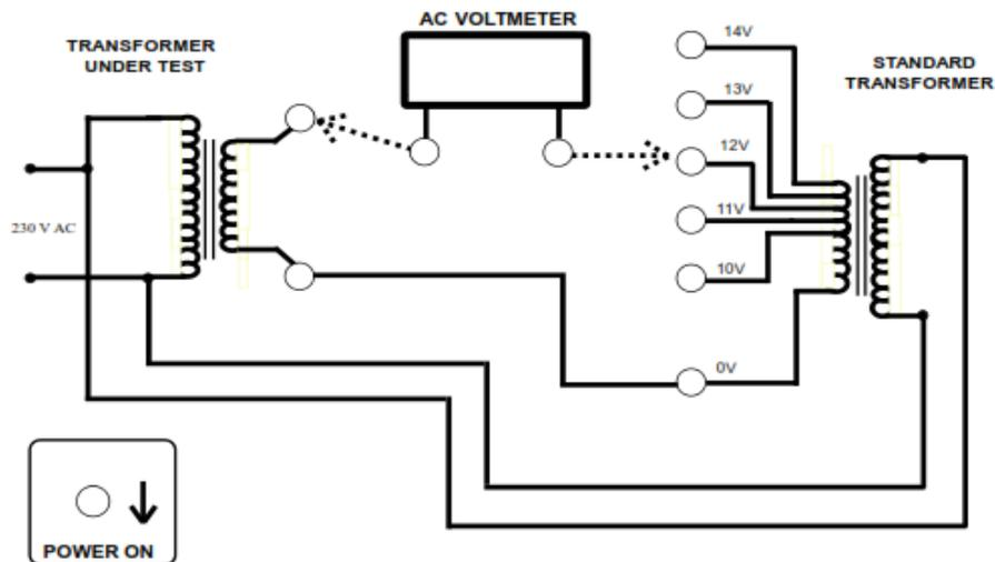
Fig -7.1 Turns Ratio Diagram
