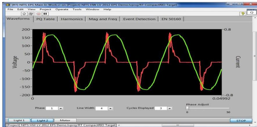
**Fig - 12.11 Design a LabVIEW front panel to display waveform data and power calculation results.**
