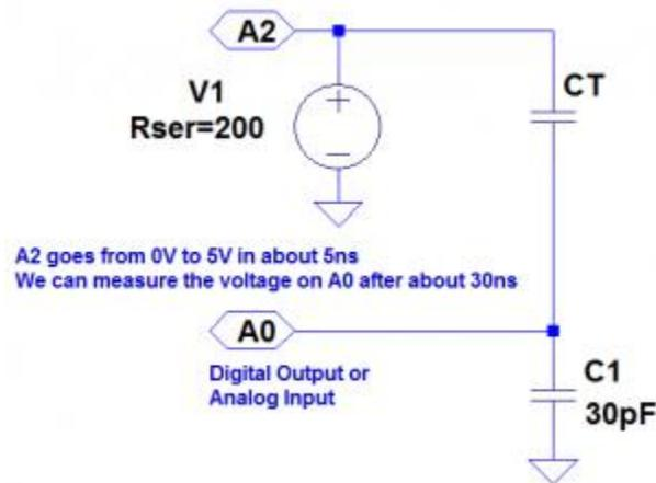
Fig – 14.12 Simulation Circuit
