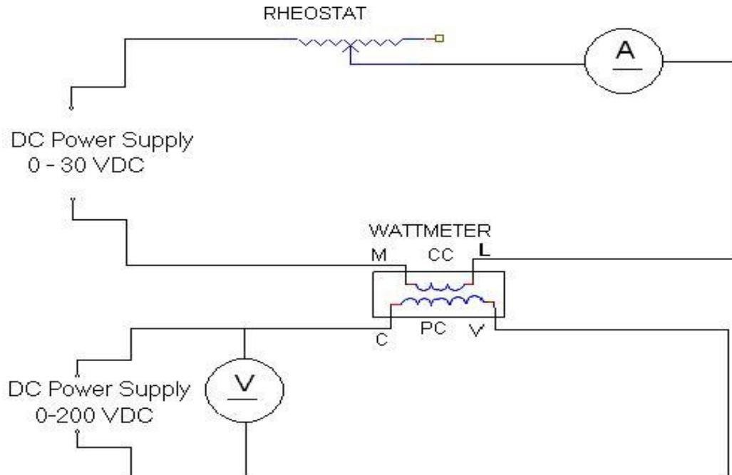
**Fig – 5.1 Calibration of LPF Wattmeter by Phantom Testing**
