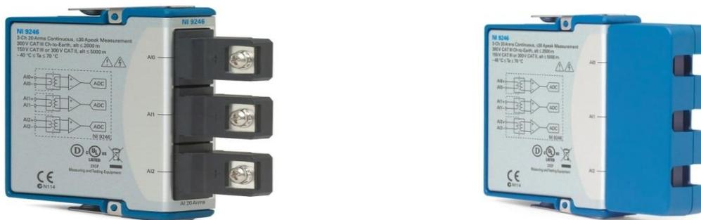
**Figure - 12.2 The NI 9246 and NI 9247 modules have CTs built into the module, large over-current ratings, and accommodate up to 10AWG wire with ring lugs for higher current measurement. Direct measurements with these modules will be more accurate and with a higher frequency response than using most external CTs/sensors. Both modules can withstand 500 ARMS for 1 second and 1250 ARMS for 1 cycle.**
