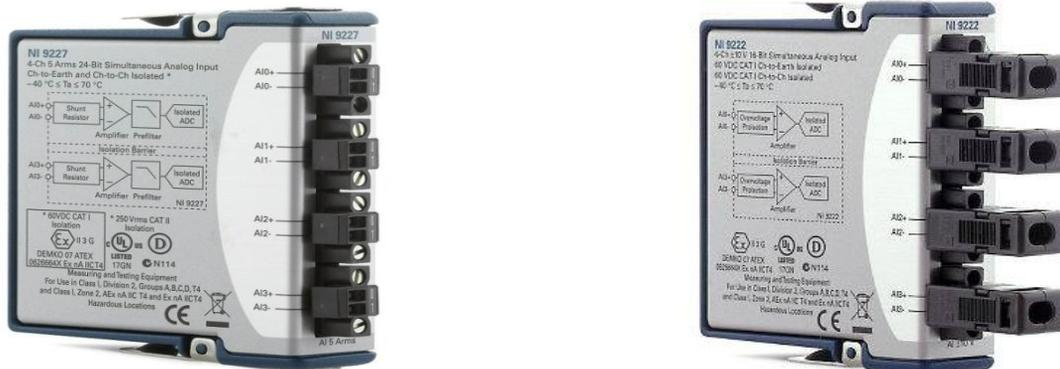
**Figure - 12.1 The NI 9229, NI 9239, NI 9227, and NI 9238 have a two terminal connector (left) for each measurement channel. Shields are available (right), and recommended, for strain relief and operator keep-outs from connections to active circuits.**
