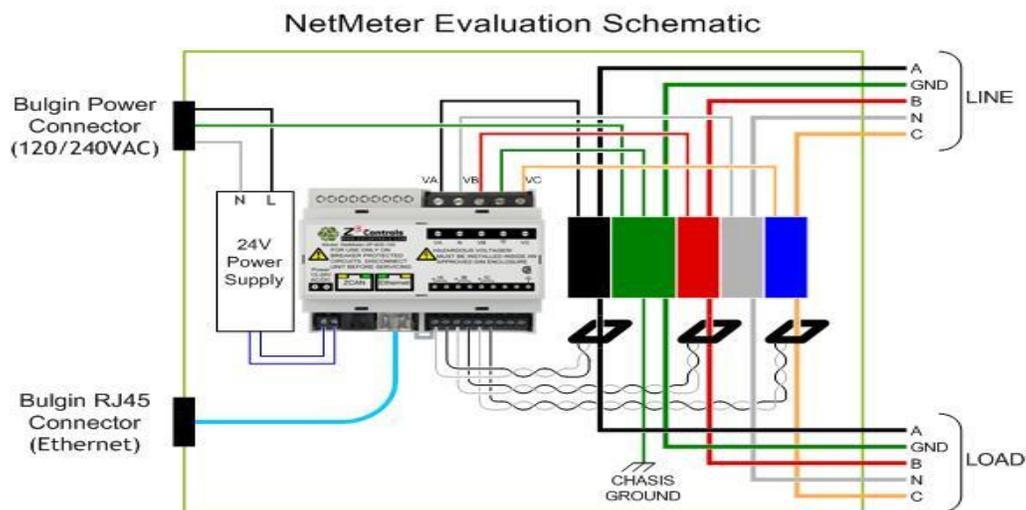
Fig – 9.2 Net Meter Evaluation Schematic
