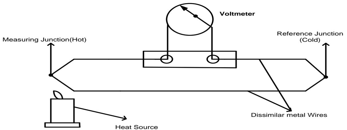
**Fig – 1.1 Thermocouple**
