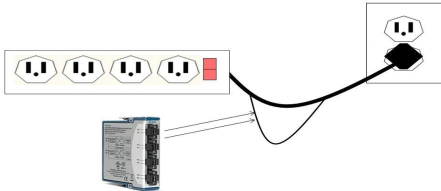
**Figure – 12.3 For direct module connection, the load wire (black in the US), is cut and connected to the AI+ and AI- terminals of a single channel. Current passing through the module is measured. In the image above with the splice in the cable, the module will measure the current flowing to all devices plugged into the power strip.**
