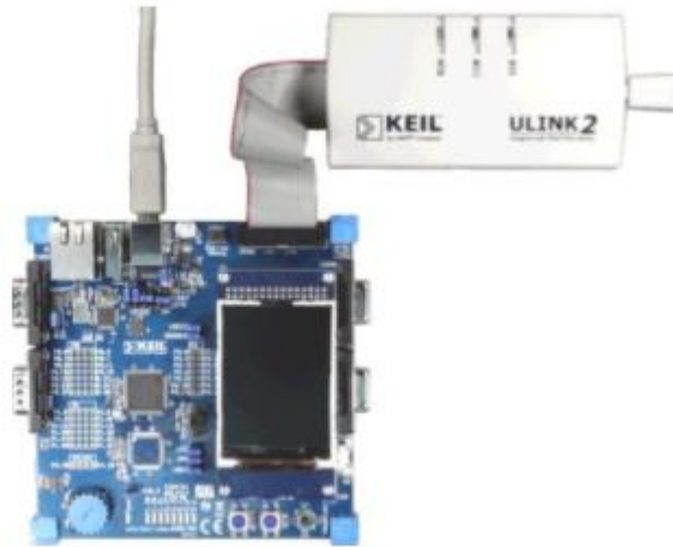
Figure 1 Connection of ULINK2 to the board.
