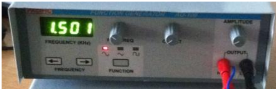
d) Function generator (input signal frequency at 1500Hz)
