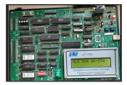
**PIC**: Programmable Interrupt controller using 8253A provides interrupts Vectors for 8 jumpers' selectable Internal /External sources.
