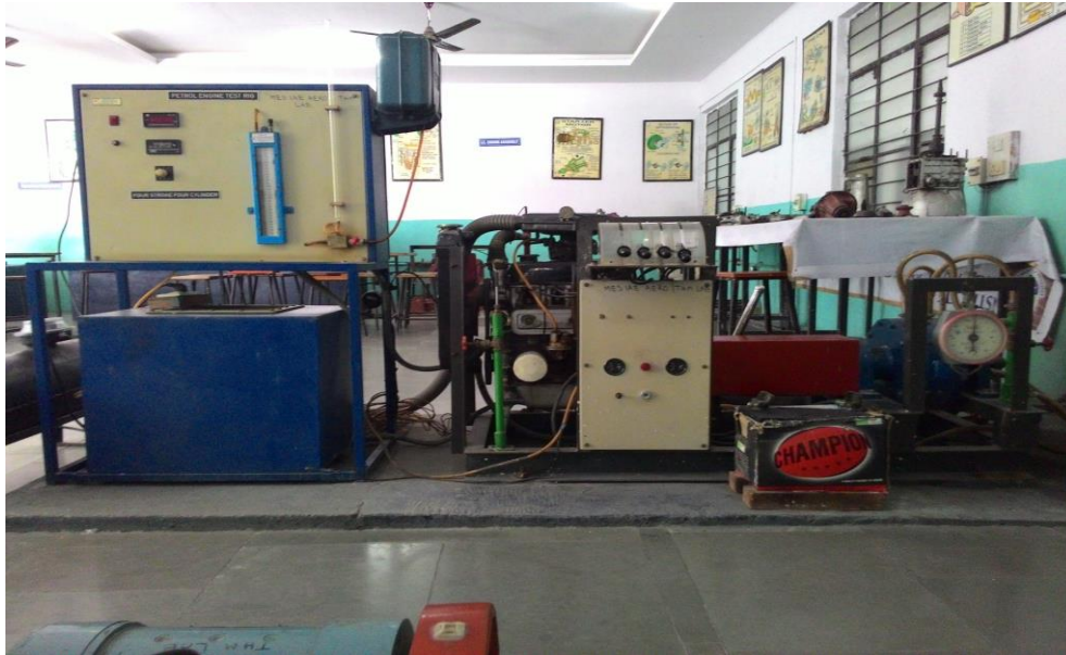
I C Engine Morse Retardation Motoring Tests
