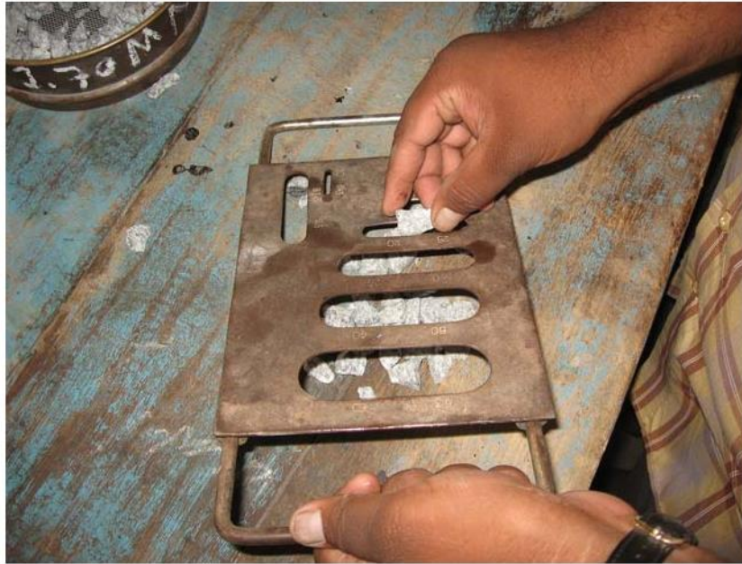
Flakiness Index Test in Progress
