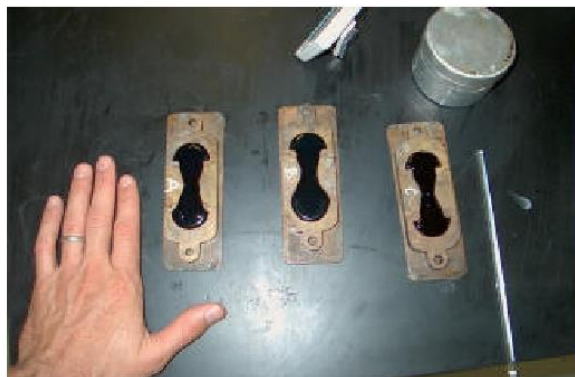
Sample Prepared in Briquette Mould and Ductility Apparatus
