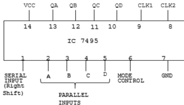
1) SERIAL IN SERIAL OUT (SISO) (Right Shift)
