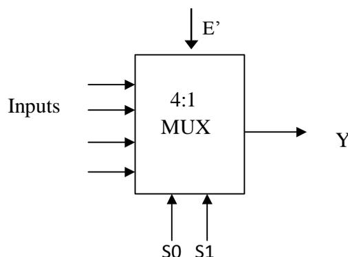
$$\text{Output } Y = E'S_1'S_0'I_0 + E'S_1'S_0I_1 + E'S_1S_0'I_2 + E'S_1S_0I_3$$
