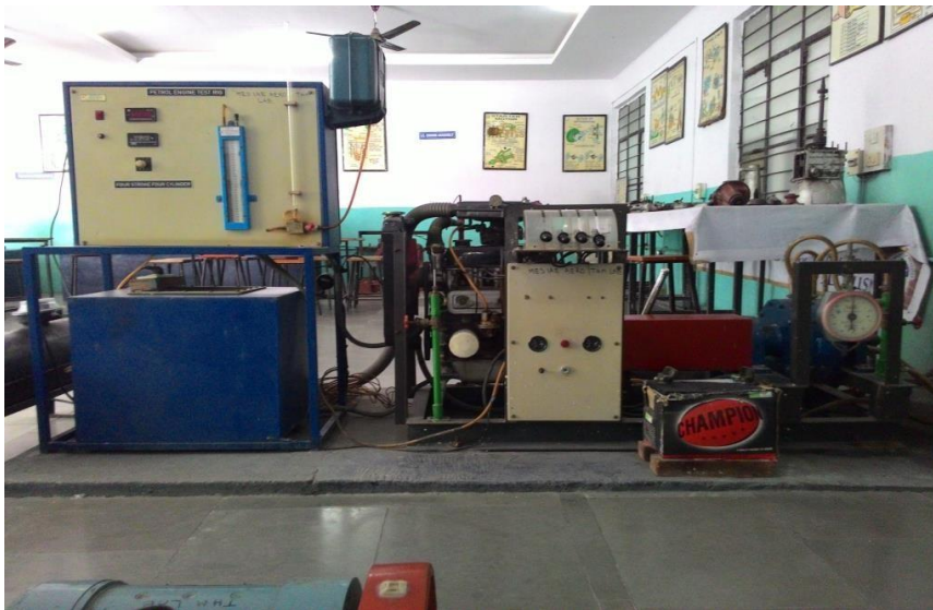
I C Engines Performance Test For 4 Stroke S I
