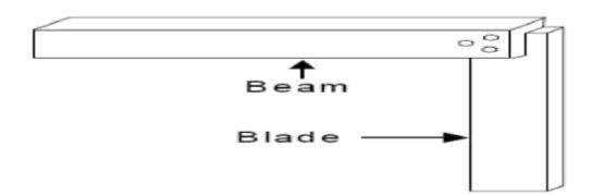
3.Marking Gauge: It is used for scoring or for folling a line parallel to a given space, edge or end. It is made of wood. There is a sharp metal spur point. Main bar of the guage has graduations printed on it similar to that of foot rule. It is always advisable to check the measurement from the spur point to movable head.
