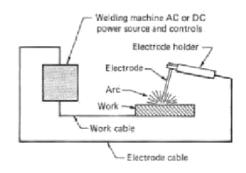
brought into the contact with the work then welding will takes place.
