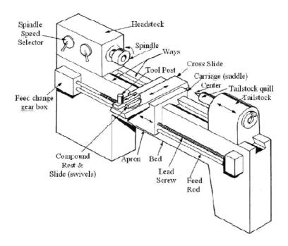
A lathe s a machine tool which rotates the workpiece on its axis to perform various operations such as cutting, sanding, knurling, drilling, or deformation with tools that are applied to the workpiece to create an object which has symmetry about an axis of rotation.
