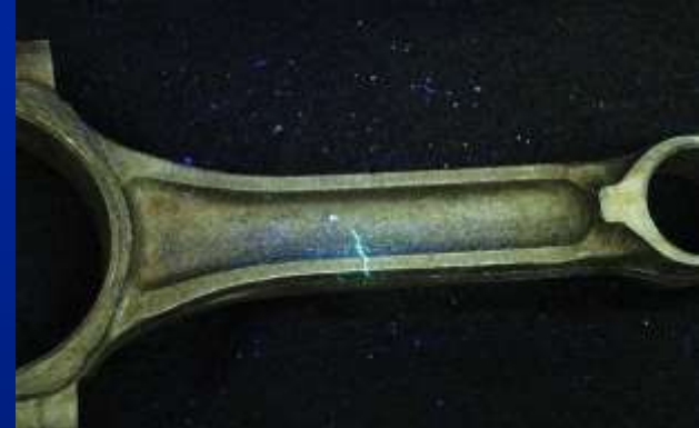
Fluorescent penetrant indication
