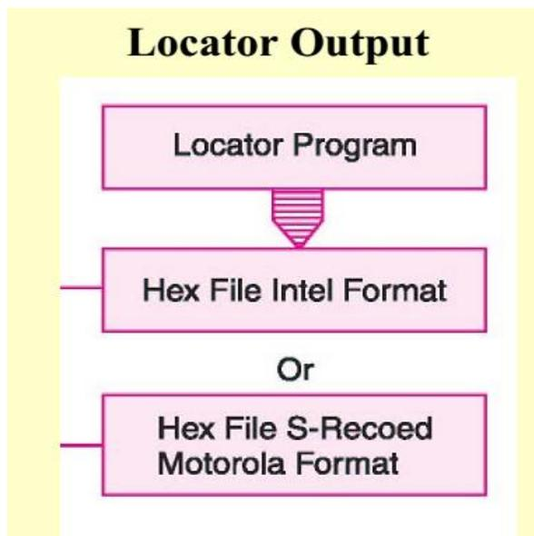
Locator includes a mechanism for programmer to determine placement in memory
