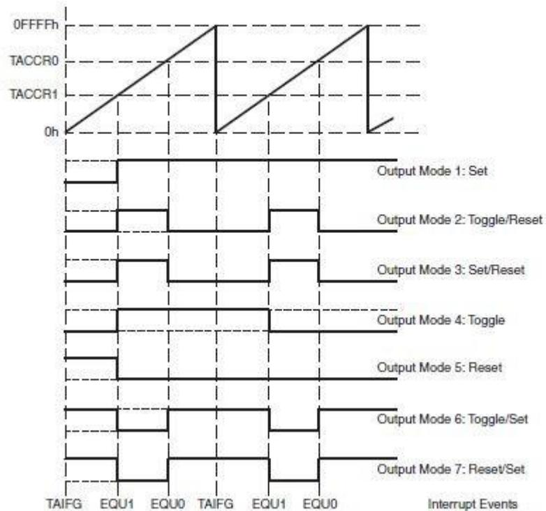
Figure 12-13. Output Example—Timer in Continuous Mode
