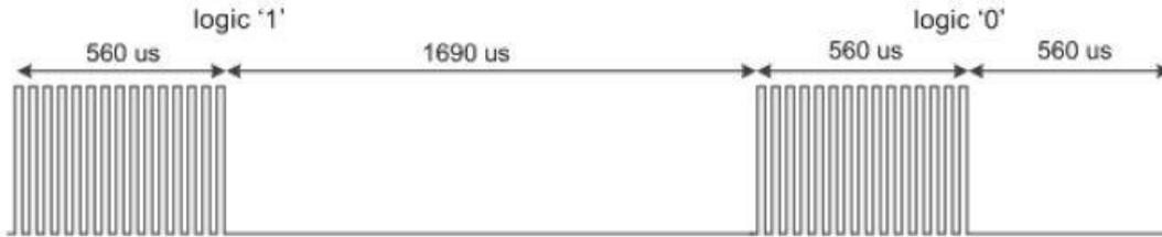
Figure 4. Pulse Distance Protocol, Bit Encoding
