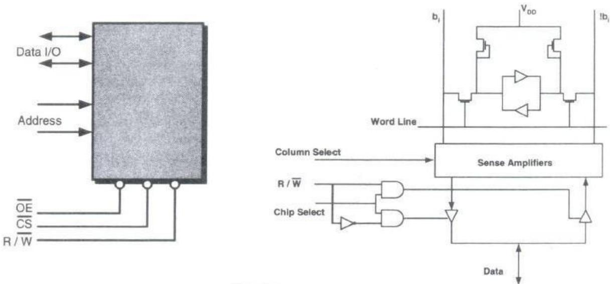
Figure 3.4 The SRAM – inside and outside
