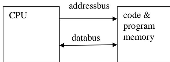
Von-Neumann architecture supports simple hardware. It allows the use of a single, sequential memory. Today's processing speeds vastly outpace memory access times, and we employ a very fast but small amount of memory (cache) local to the processor.
