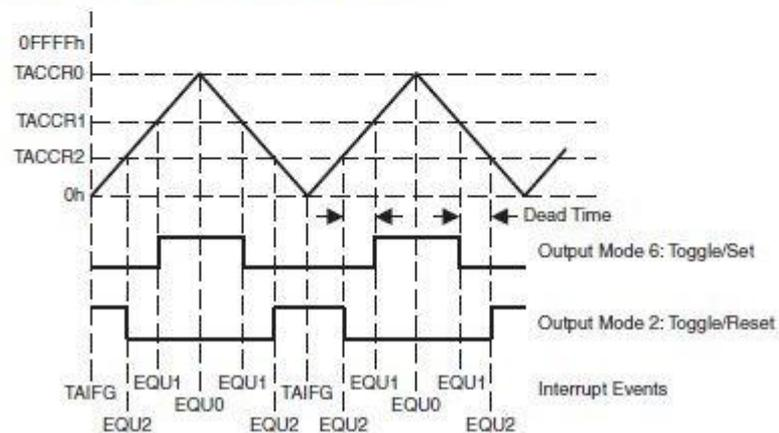
Figure 12-9. Output Unit in Up/Down Mode
