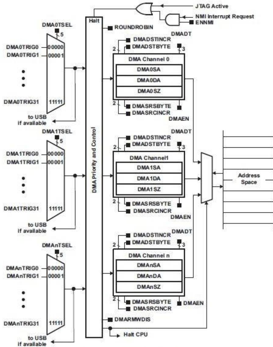
Figure 9-1. DMA Controller Block Diagram
