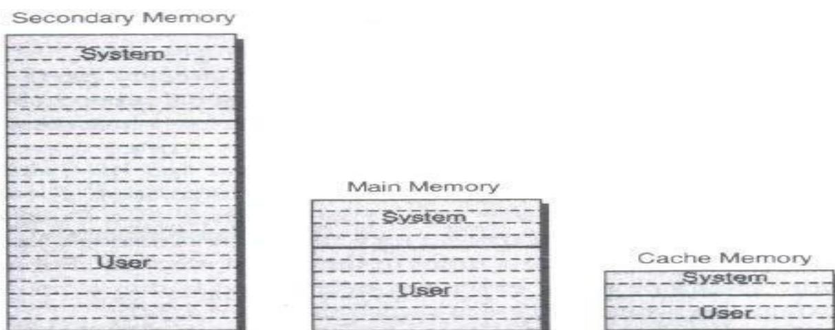
Figure 3.12 : Typical memory hierarchy utilizing a variety of memory types.
