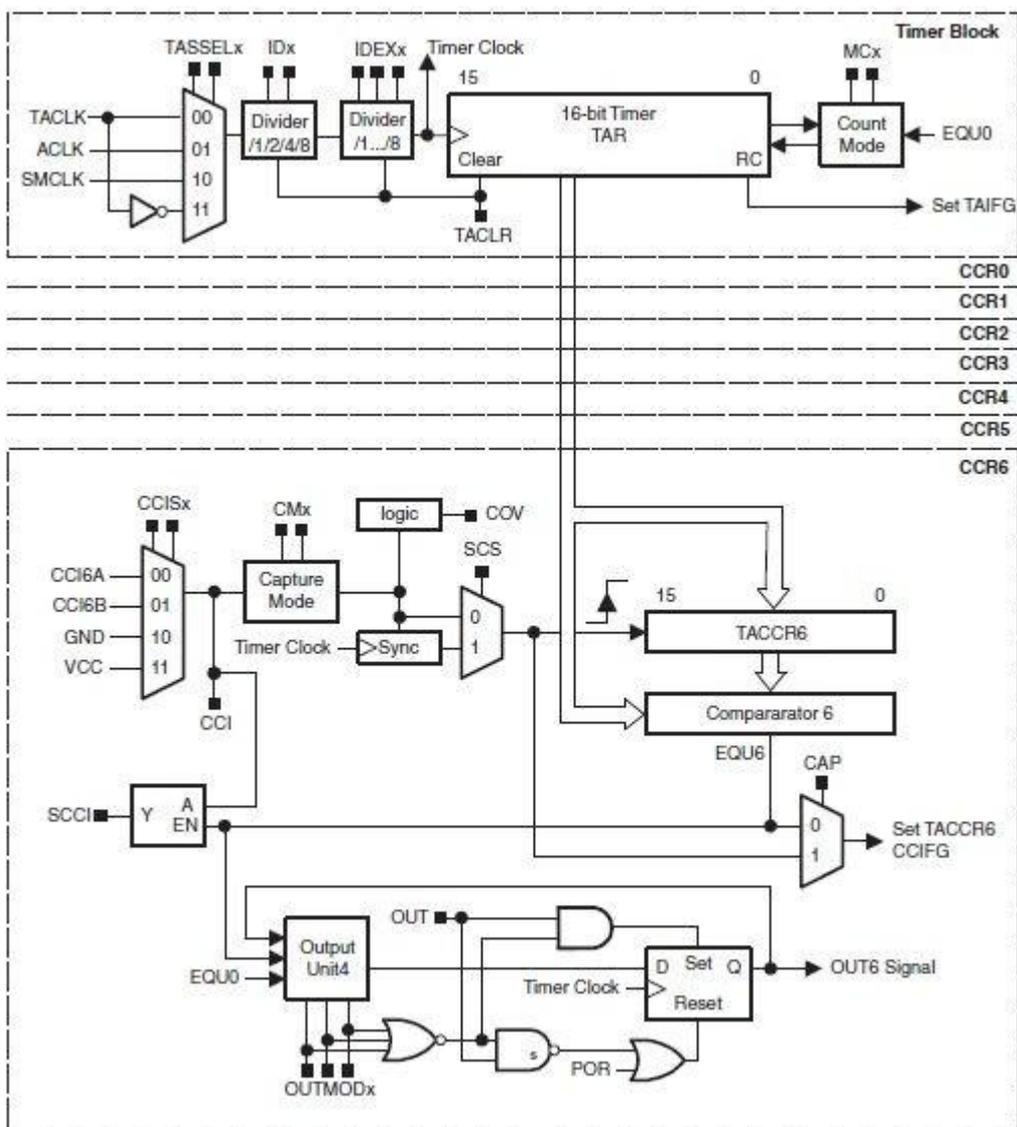
The 16-bit timer/counter register, TAR, increments or decrements (depending on mode of operation) with each rising edge of the clock signal. TAR can be read or written with software. Additionally, the timer can generate an interrupt when it overflows.
