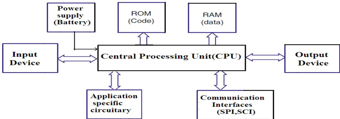
**Fig: hardware architecture of embedded system**
