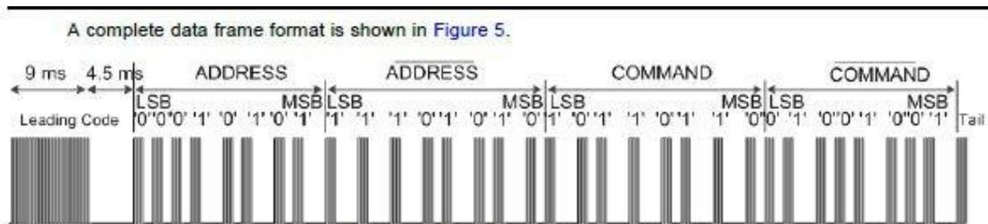
Figure 5. Pulse Distance Protocol, Data Frame Format
