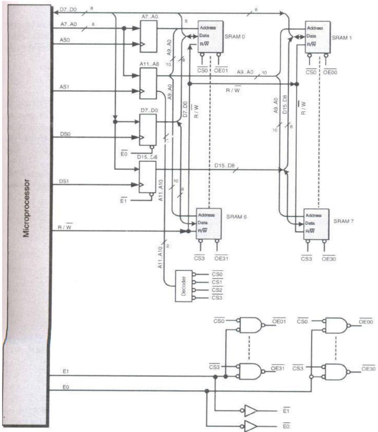
Figure 3.9: Design a 4K \* 16 SRAM system
