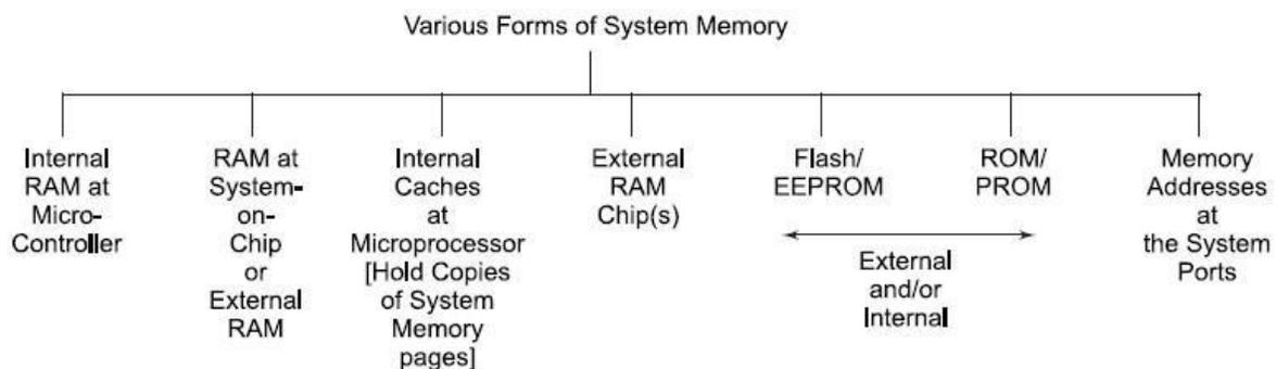
Table 1.1 gives the functions assigned in the embedded systems to the memories. ROM or PROM or EPROM embeds the embedded software specific to the system.
