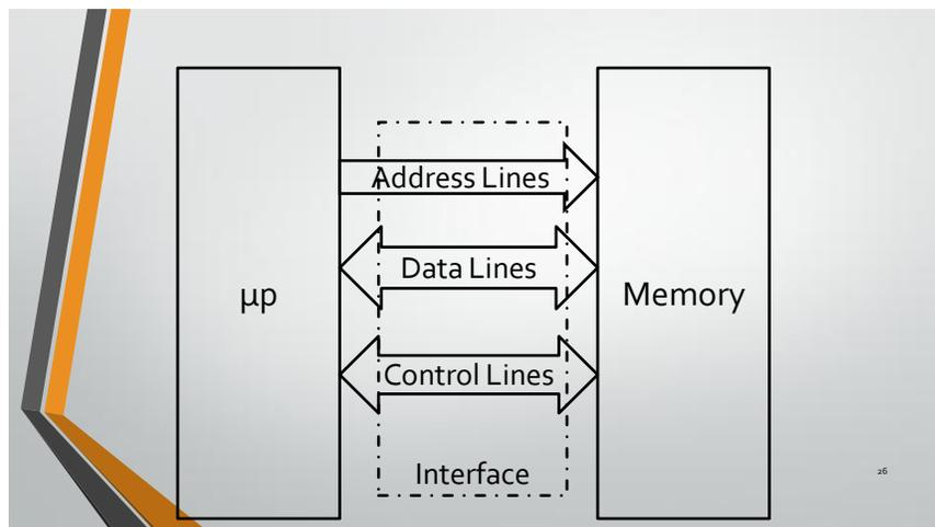
In parallel I/O have two types of interfacing
