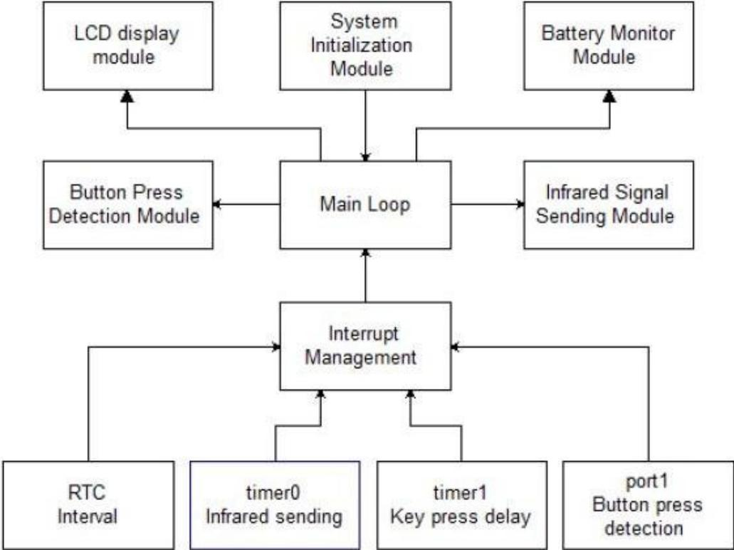
Figure 3. Software Structure
