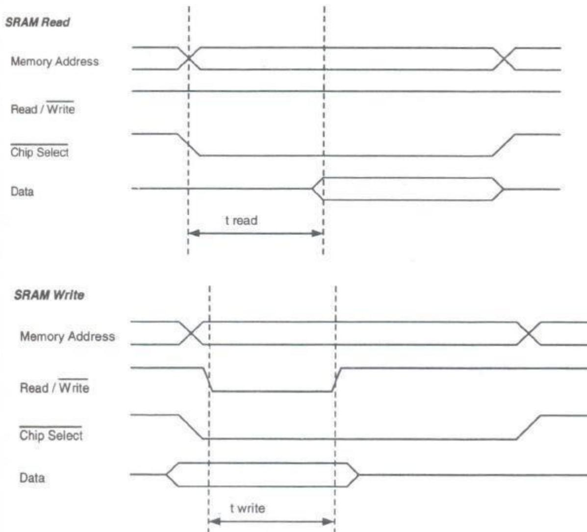
Figure 3.5 timing for the SRAM-read and write operation
