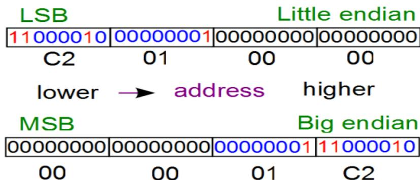
Big endian systems are simply those systems whose memories are organized with the most significant digits or bytes of a number or series of numbers in the upper left corner of a memory page and the least significant in the lower right, just as in a normal spreadsheet.
