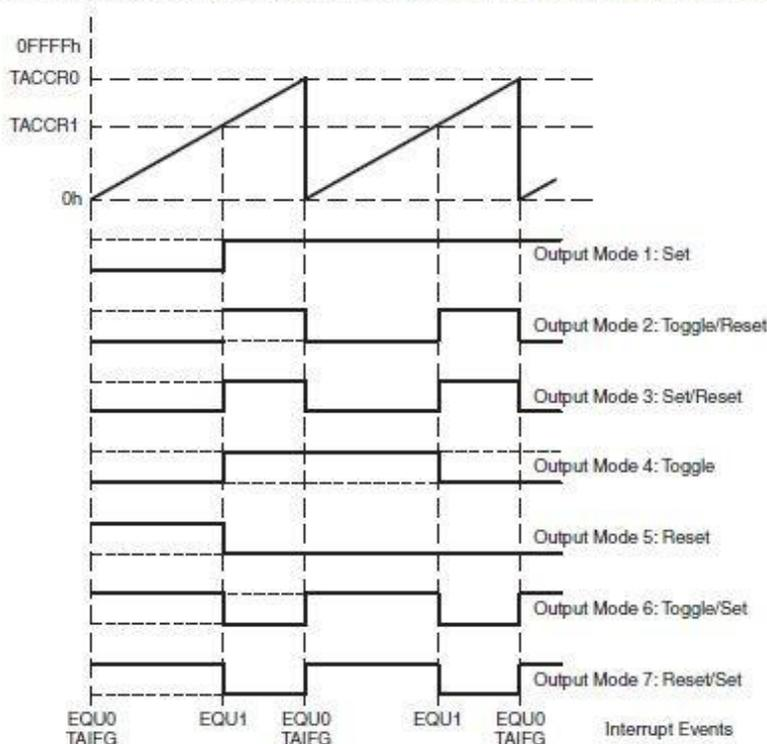
Figure 12-12. Output Example—Timer in Up Mode
