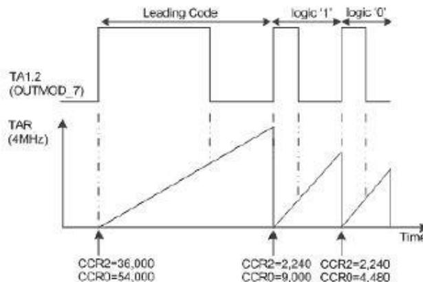
Figure 6. Pulse Distance Protocol, TA1 in Envelope Generation
