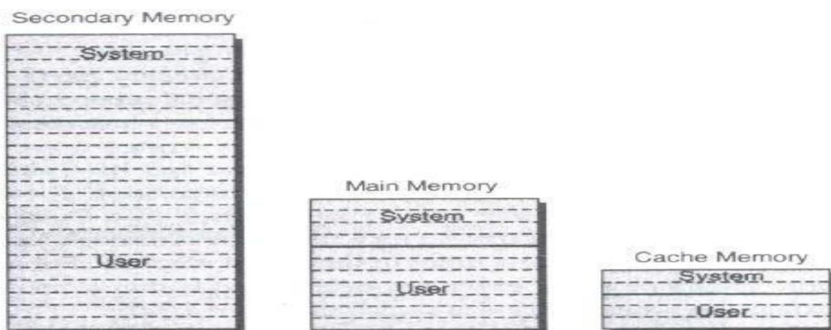
Figure 3.12 : Typical memory hierarchy utilizing a variety of memory types.
