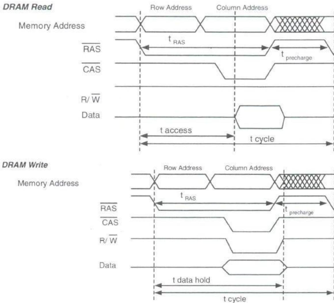
Figure 3.7 : Timing for the DRAM read and write cycles
