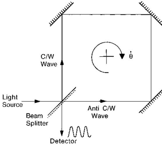
Sagnac interferometer. The clockwise and anti-clockwise waves interfere to produce a fringe pattern which shifts when the interferometer is subjected to input rate,  $\dot{\theta}$ .
