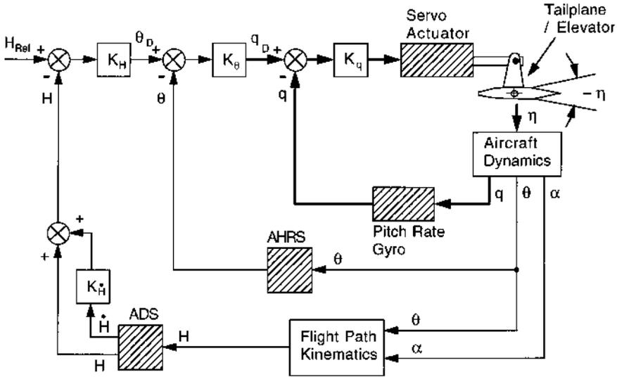
Height control (heavy lines show FBW pitch rate command loop). Pitch rate gyro and AHRS are shown separately for clarity. In a modern aircraft, a strap-down AHRS/INS provides both  $\theta$  and  $q$  outputs.
