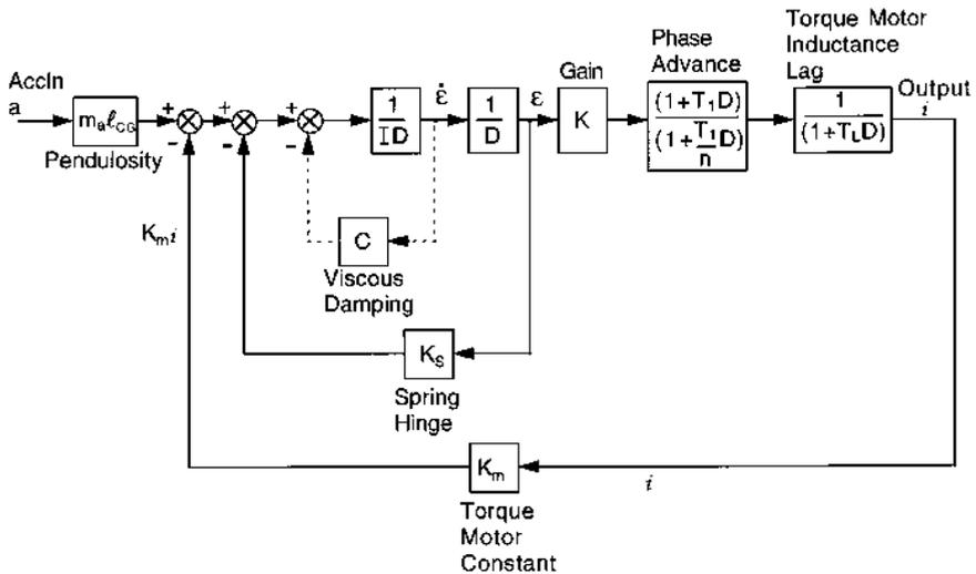
Torque balance accelerometer loop.
