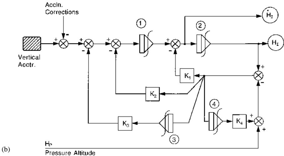
(a) Baro-inertial mixing. Simple second-order baro-inertial mixing shown in bold lines. Integral term correction for inertial drift shown in dotted lines. (b) Fourth-order baro-inertial mixing (with correction for inertial channel drift and pressure altitude error).
