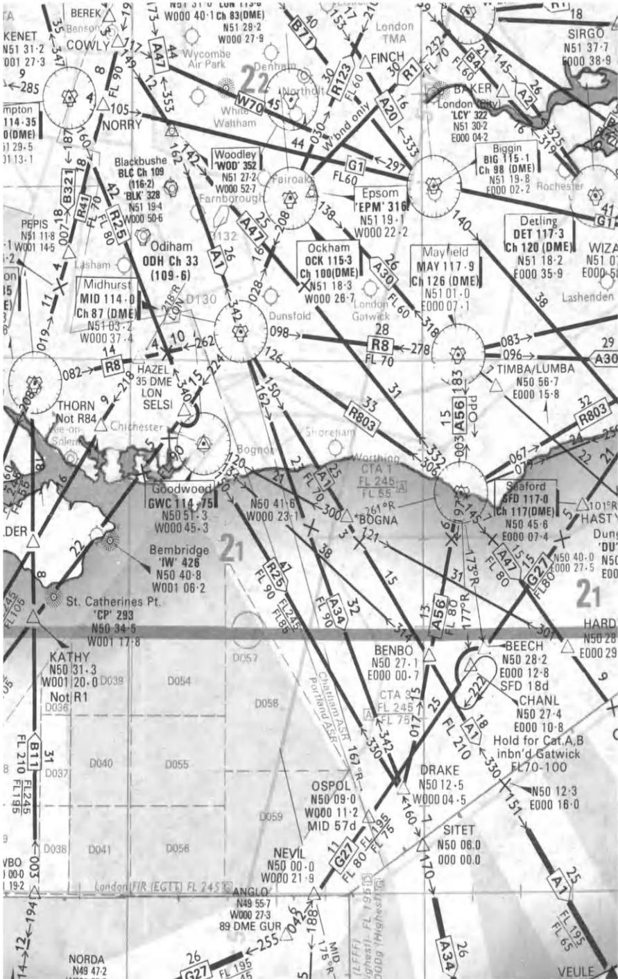
Section of radio navigation chart (by courtesy of British Airways AERAD).
