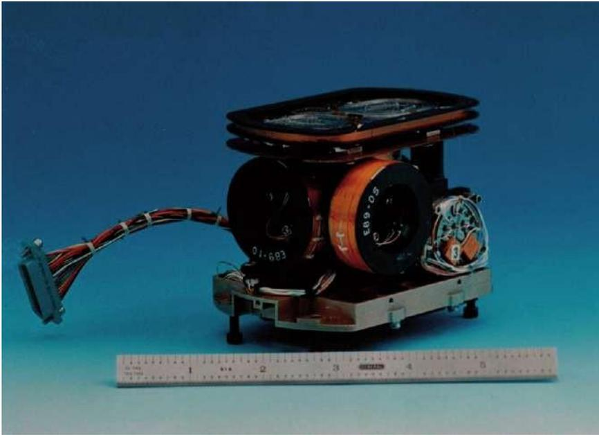
Fibre optic gyro inertial measuring unit (courtesy of Smiths Industries).
