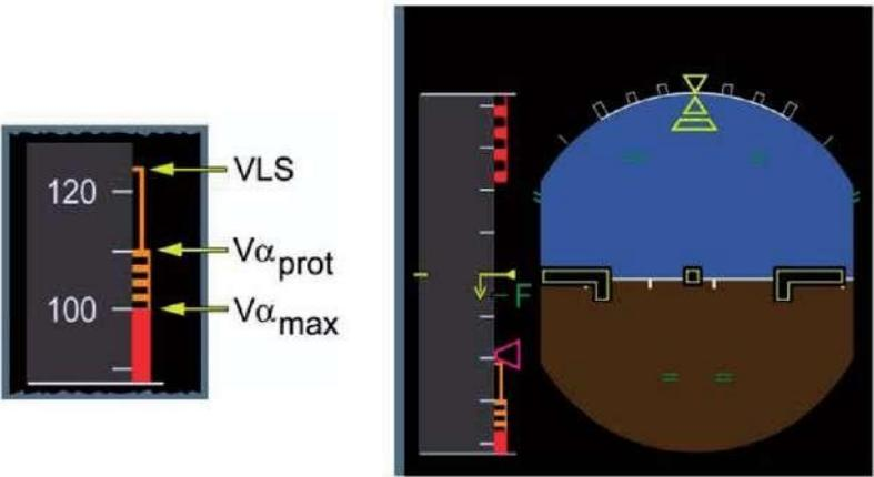
Speed scale showing safe limiting values on PFD (by courtesy of Airbus).
