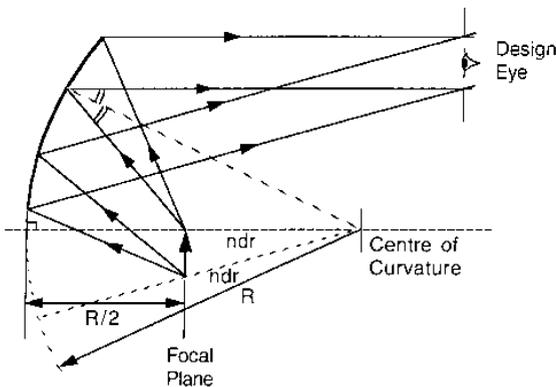
Collimation by a spherical reflecting surface.
