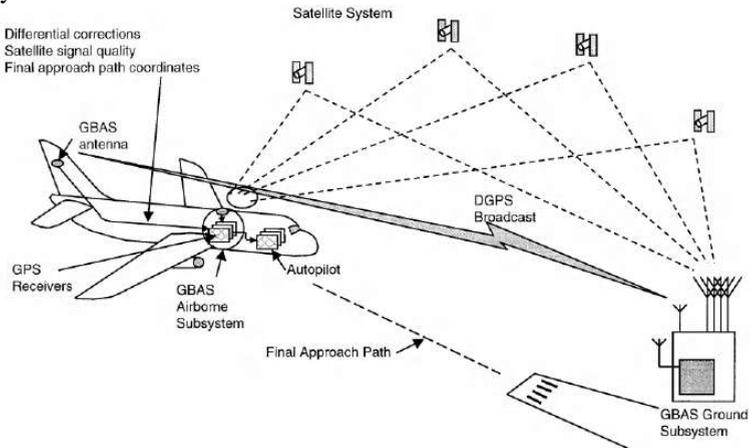
The flight path kinematics to align the aircraft's flight path with the commanded flight path are the same whether this is defined by a radio/microwave beam or the GBAS
