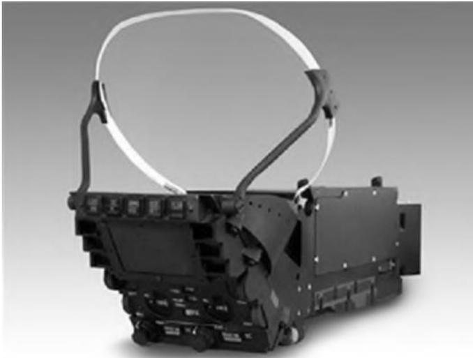
Wide FOV holographic HUD installed in Eurofighter Typhoon (by courtesy of BAE Systems).
