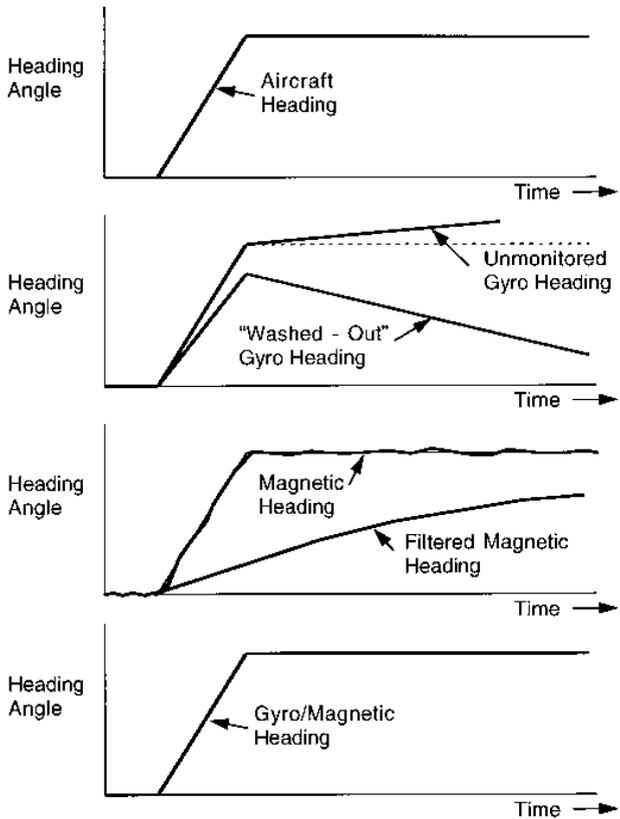
Complementary filtered gyro/magnetic heading response to constant rate of turn.
