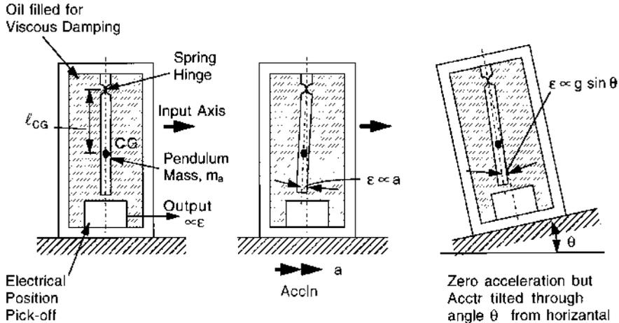
Simple spring restrained pendulous accelerometer.
