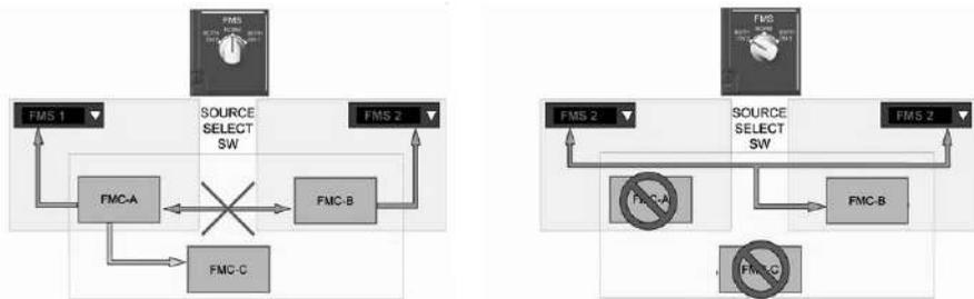
Independent Mode and Single Mode configurations (by courtesy of Airbus).
