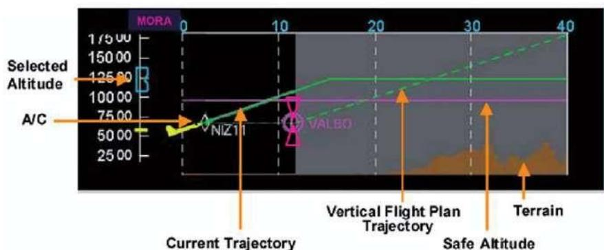
Aircraft trajectory in vertical plane displayed on lower section of Navigation Display (by courtesy of Airbus).
