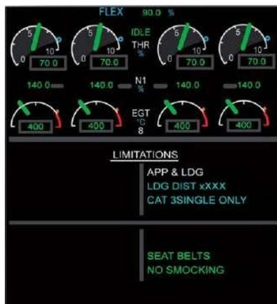
Engine/Warning display (by courtesy of Airbus).
