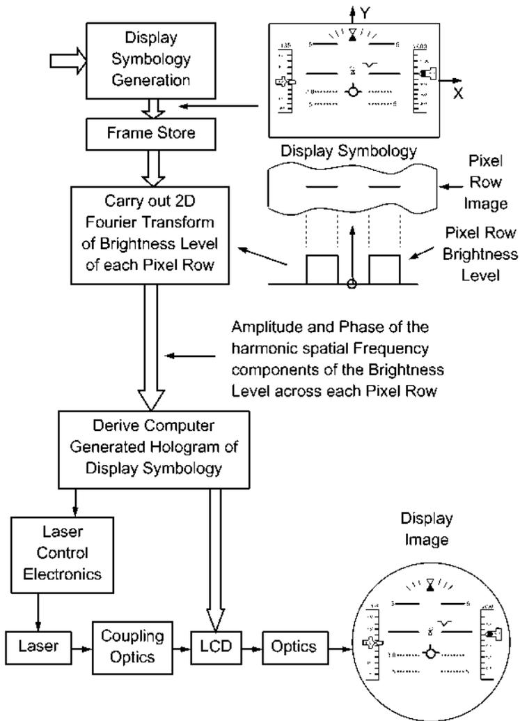
Block diagram of active CGH method of generating a fault tolerant display.
