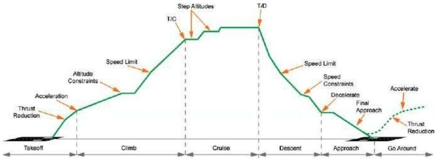
Flight plan – vertical definition (by courtesy of Airbus).
