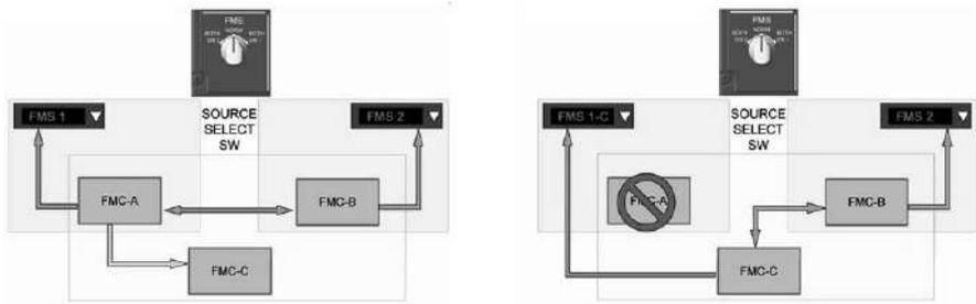
Dual Mode operation (by courtesy of Airbus).
