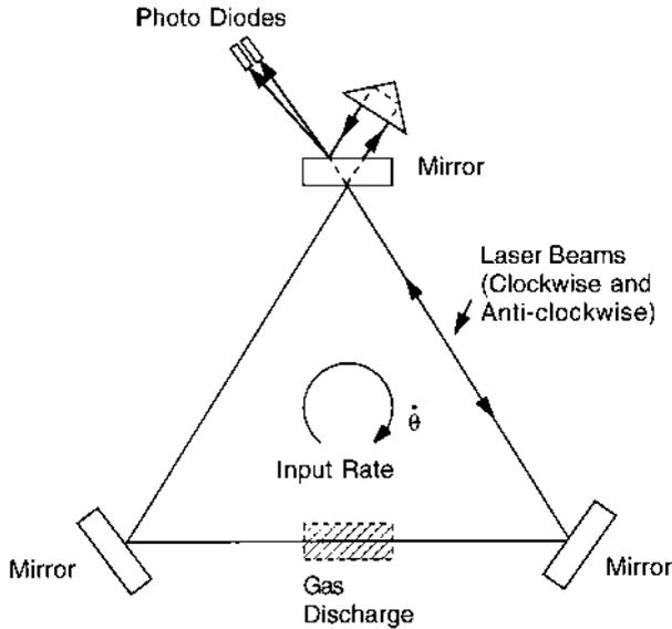
Laser gyro schematic.
