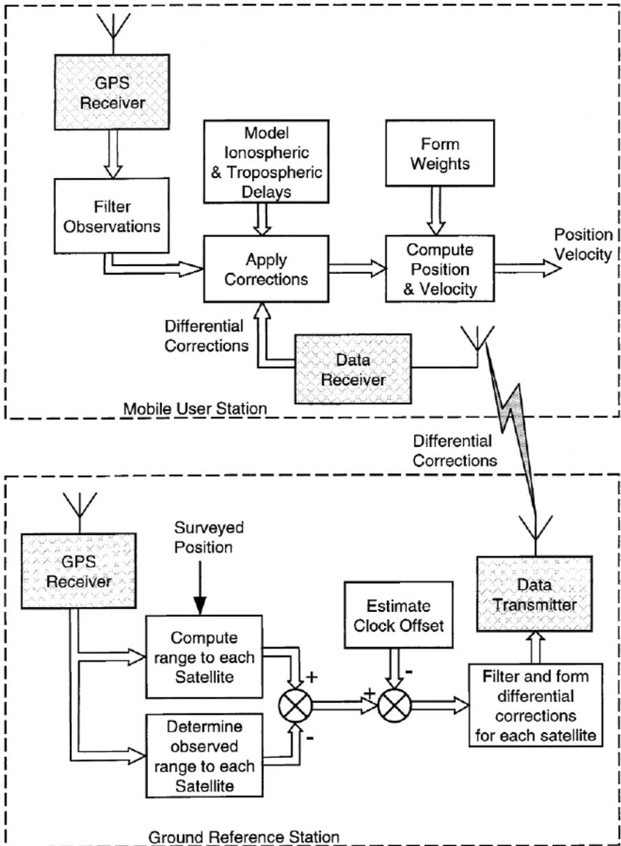
Simplified functional diagram of a generic differential GPS system.
