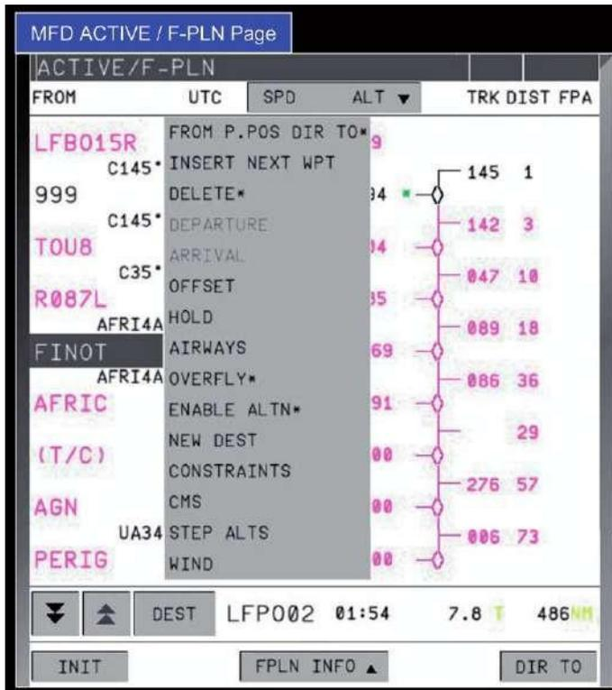
‘Active Flight Plan’ Page display on MFD (by courtesy of Airbus).
