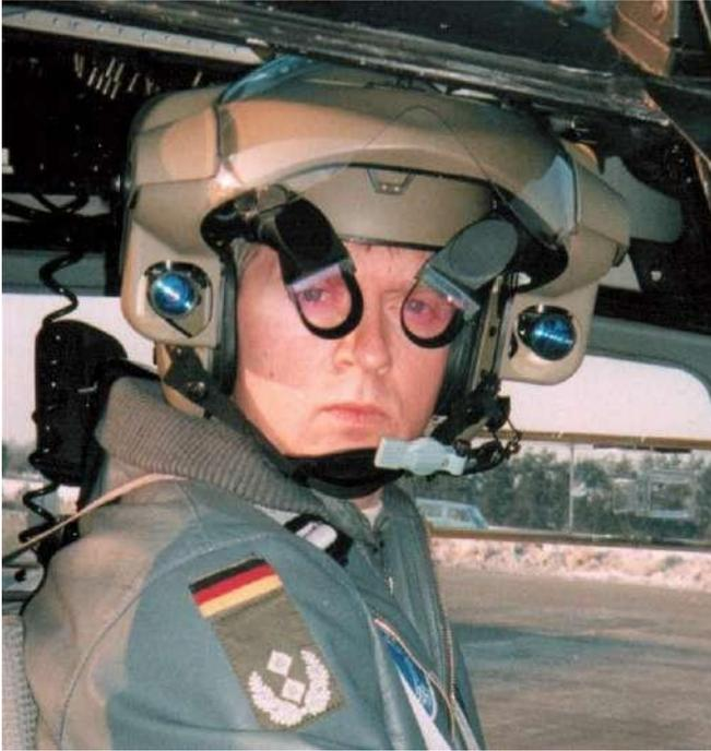
Helicopter HMD with integrated NVGs (by courtesy of BAE Systems). This HMD forms part of the mission systems avionics for the Tiger 2 attack helicopter for the German army.
