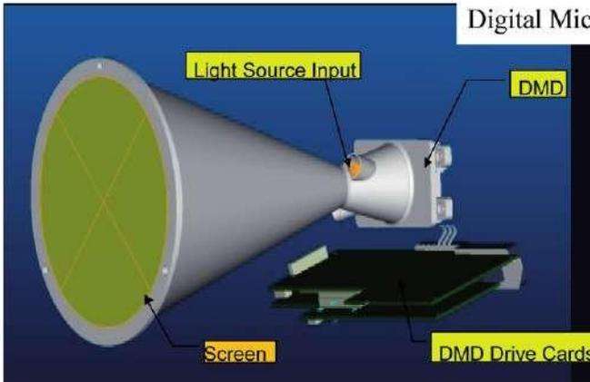
'Digital Light Engine' projector display unit (by courtesy of BAE Systems).
