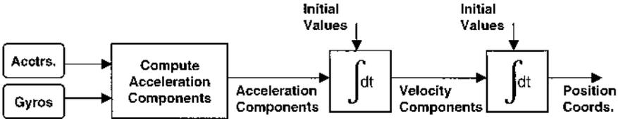
Basic principles of inertial navigation.
