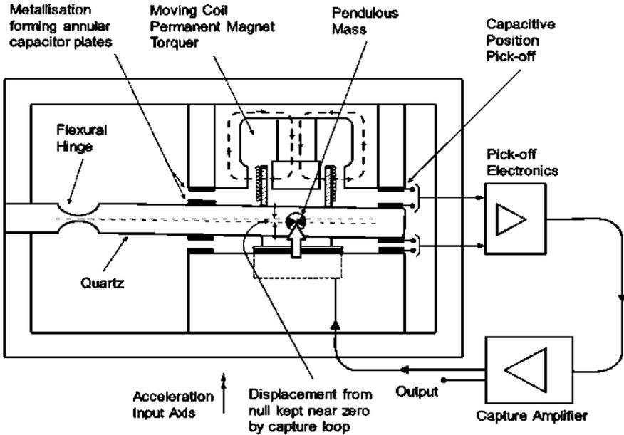
Torque balance pendulous accelerometer schematic.
