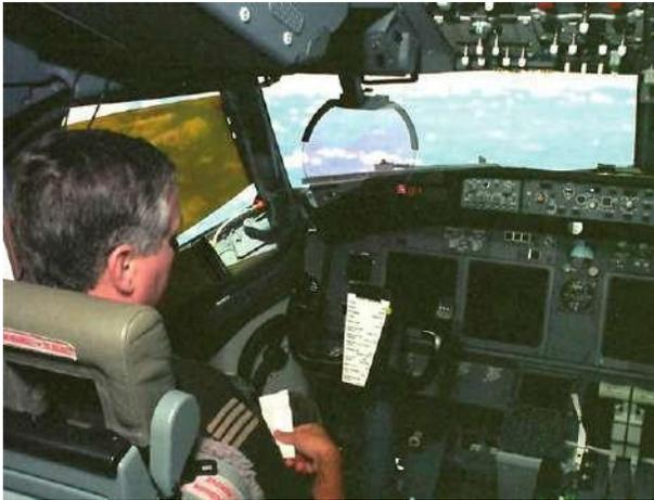
Civil HUD installation – BAE Systems VGS HUD installed in a Boeing 737-800 series airliner (by courtesy of BAE Systems).
