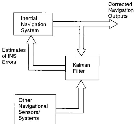
Block diagram of aided IN system with Kalman filter.
