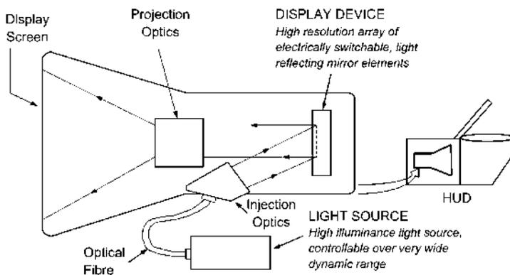
Block diagram of a HUD projected display unit.
