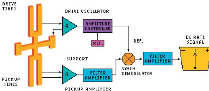
Quartz rate sensor (courtesy of Systron Donner Inertial Division).
