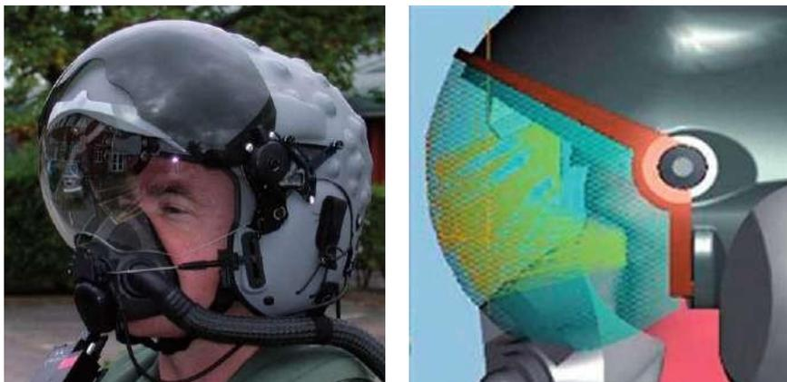
Eurofighter Typhoon binocular visor projected HMD (by courtesy of BAE Systems). Right side illustration shows optical ray trace. Displays images are collimated by reflection from the spherical visor. Note use of 'brow' mirror to relay display images.
