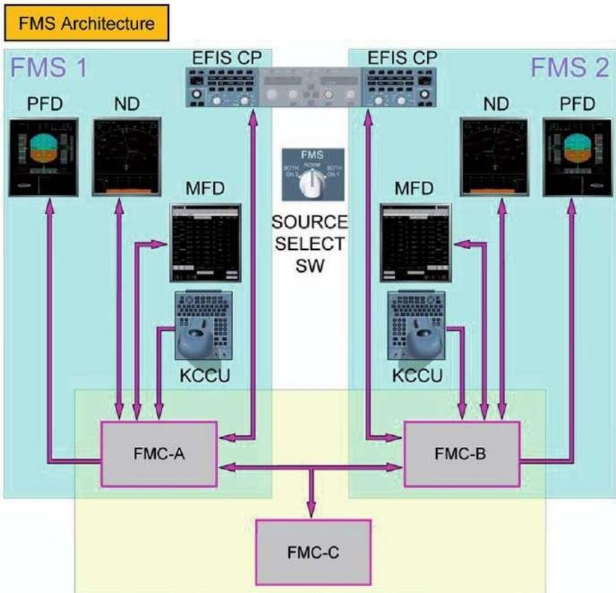
FMS architecture (by courtesy of Airbus).
