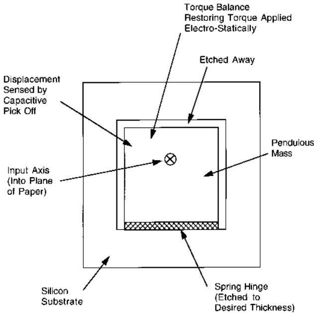
'Solid state' dry accelerometer construction.
