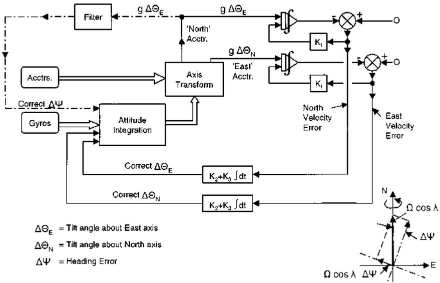
Fine levelling and gyro compassing loops.
