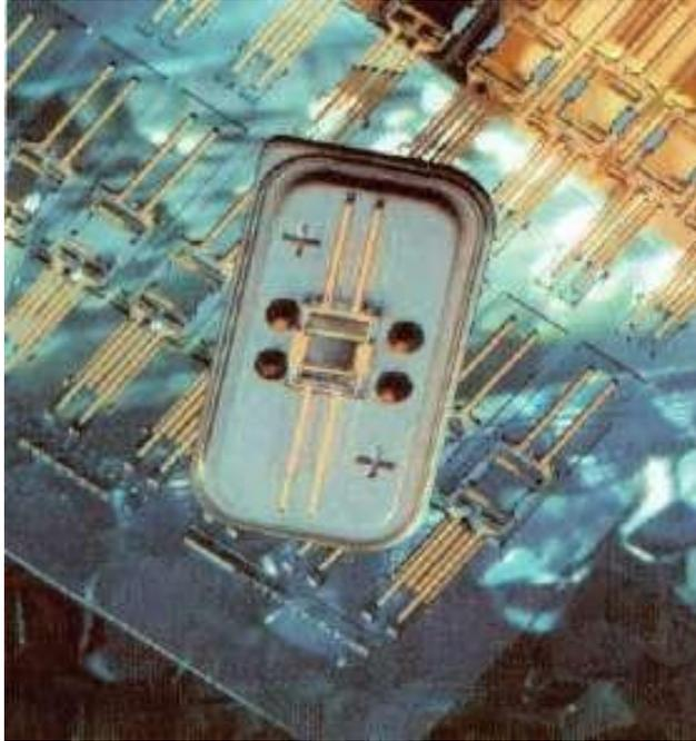
Quartz rate sensor fabrication wafer with device overlaid (courtesy of Systron Donner Inertial Division).
