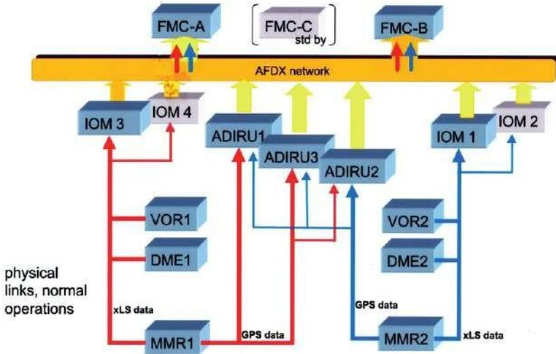
Interconnection of Navigation System units by the AFDX network (by courtesy of Air-bus).
