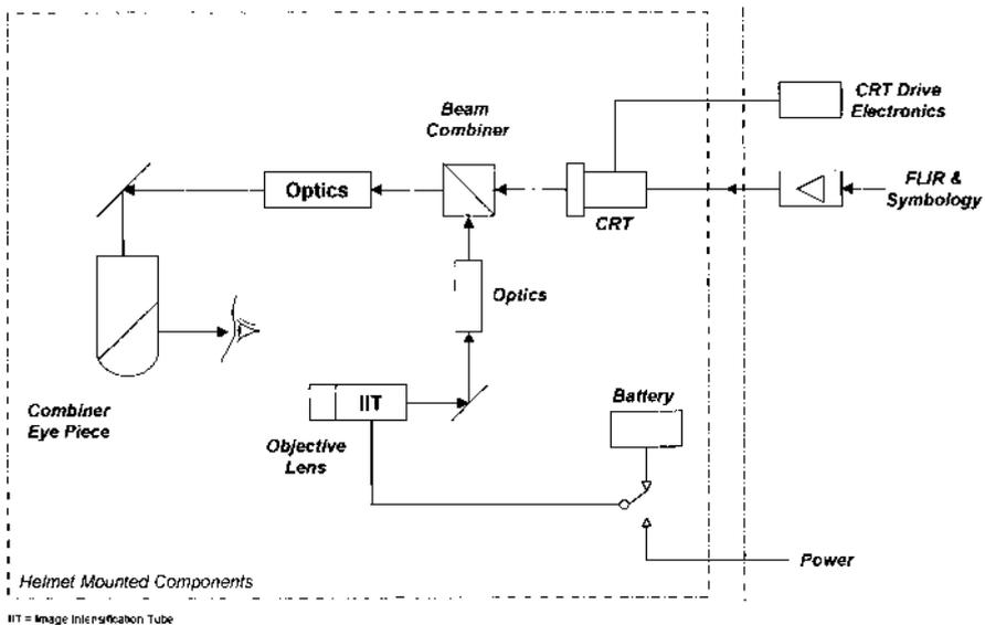
Optical mixing of IIT and CRT imagery.
