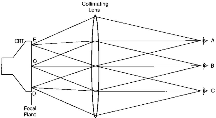
Simple optical collimator ray trace.
