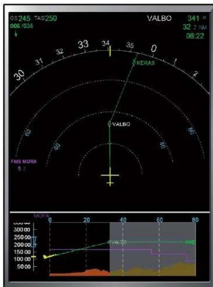
Navigation (or horizontal situation) displays (by courtesy of Airbus).
