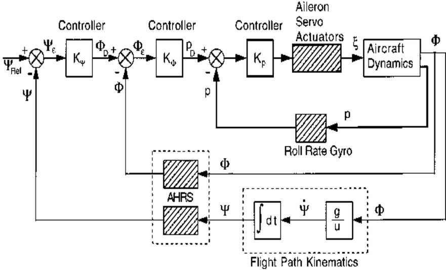
Heading control loop (heavy lines show FBW roll rate command loop). Roll rate gyro and AHRS are shown separately for clarity. In a modern aircraft, a strap-down AHRS/INS provides both  $p$  and  $\delta$  outputs.
