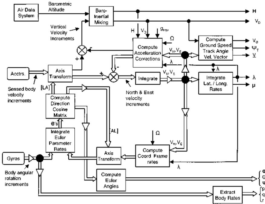
Strap-down INS computing flow diagram.
