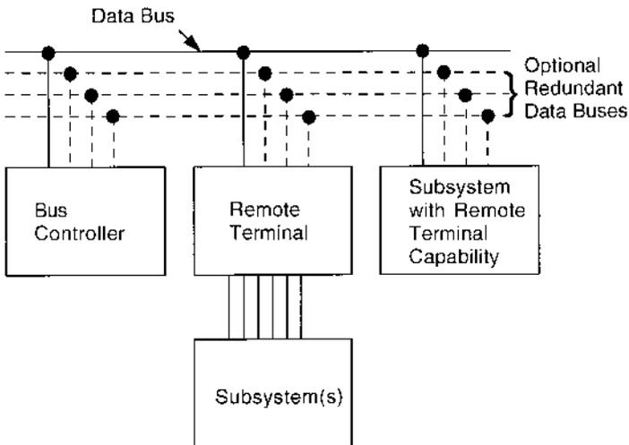
Typical multiplex data bus system architecture.
