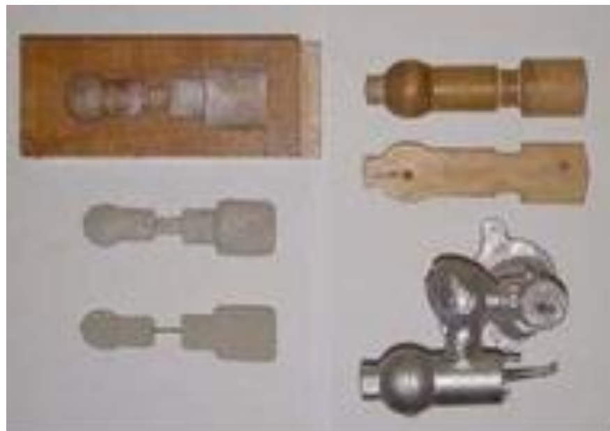
FIGURE - Left: - Core box, with resulting (wire reinforced) cores directly below. Right: - Pattern (used with the core) and the resulting casting below (the wires are from the remains of the core). After casting, the cores are broken up by rods or shot and removed from the casting. The metal from the sprue and risers is cut from the rough casting. Various heat treatments may be applied to relieve stresses
