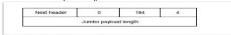
Figure: The hop-by-hop extension header for large data grams (jumbo grams)
