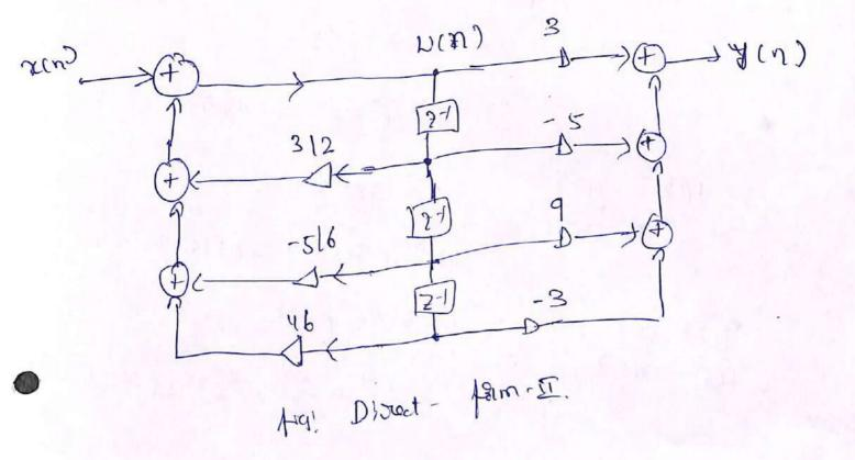
the direct form-II realizations of a discrete-Eg:- Find system represented by the transfer function. time
