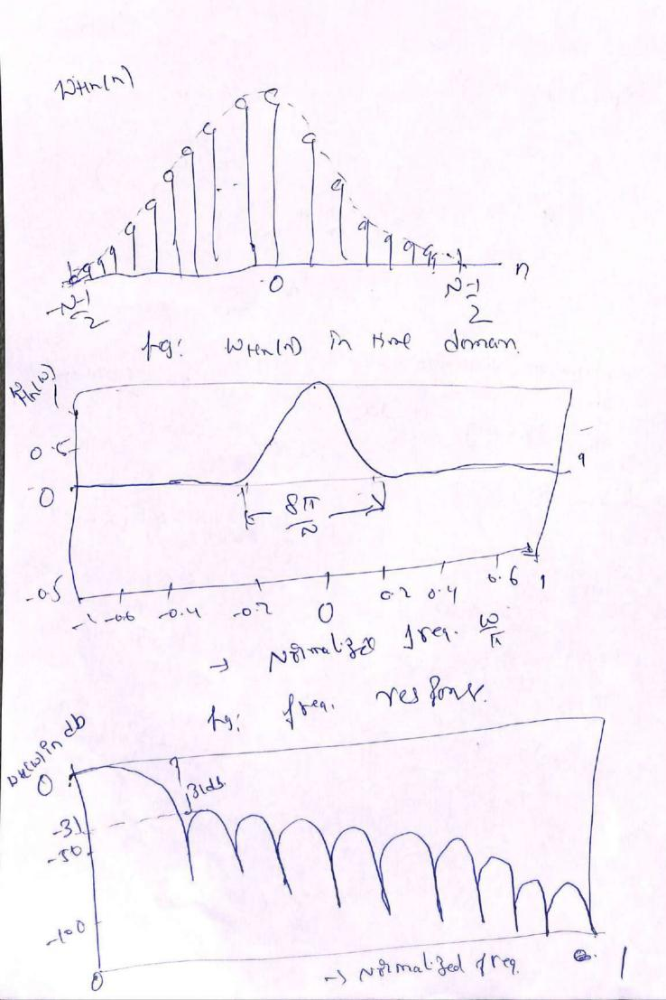
14-16 -> The men. Stop band attenuation of the filer a Len do. Hamming Mugani-Sch. 2=0.54 PM Railed cosme window DH(U) = (0.24 + 0.46 00) (200) ). A - (N-1) INI NJ freq. response of Hamming window y The HH(6)= 0.24. Sluno + 0153. Slu ( MN- MV) SINUIZ 3m ( 2 + 5.) 40.23. Sin ( WP + trip) SM ( 2 + E)
