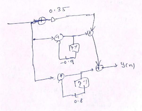
Ext. -1. Realize the system both difference can. you) = 3 yours - 1 yen-2) + xen) + 3 xen-i) in Parallel form. Sy H(2) = 60 Realise the system fiven by difference equation 2. y(n) = -0.1 y(n-1) + 6.72 y(n-2) + 0.7 k(n) - 0.25x(n-2) In Parallel four H(2) = 6.7 -0.252 2-2 1+0.1 2-1-0.729-2 = 0.35 + 0.35 - 0.035 3-1 1+0.12-1-0.722-2 - 0.35 + 0.206 + 0.14y = (+ H((2) + 4(2(2) HICE) In clinect form-12. x(cn) 0.206 41(n)
