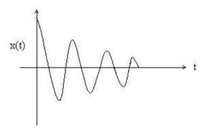
Displacement versus time in a damped oscillator
