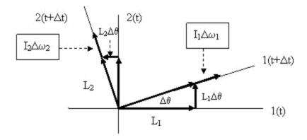
The principal axes of a rotating body at time t and  $(t+\Delta t)$ . In time interval  $\Delta t$  the body and the attached frame have rotated by an angle  $\Delta \theta$  about the z-axis and the components of angular velocity have changed by  $\Delta \varpi_1$  and  $\Delta \varpi_2$ .
