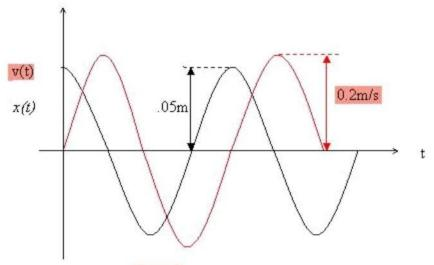
Displacement and velocity in example 1 with the initial condition x(0)=0.5m and v(0)=0.
