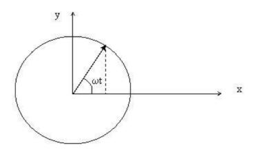
Projection of a vector  $\vec{A}$  rotating counterclockwise at a rate  $\varpi$  on the x-axis gives  $x(t) = A\cos \varpi t$
