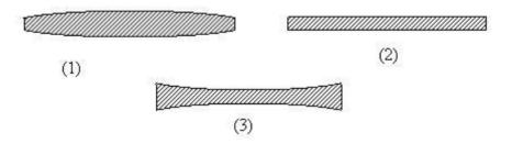
Three rollers of different shapes that are made to roll on a curved track. Only roller 1 goes over the entire track; the other two fall off it.
