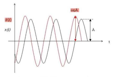
Displacement and velocity in a harmonic oscillator
