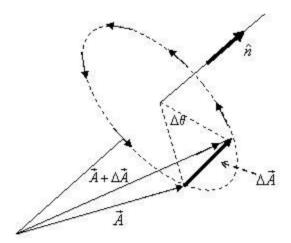
Change  $\Delta \vec{A}$  in a vector  $\vec{A}$  when it is rotated by  $\Delta \theta$  about an axis in the direction of  $\hat{n}$ .
