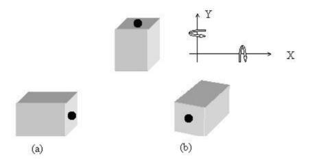
Results of two rotations – one about the x-axis by 90° counterclockwise and the second about the y-axis by 90° counterclockwise – performed on a box: (a) x-axis rotation that is followed by y-axis rotation, (b) y-axis rotation that is followed by an x-axis rotation.
