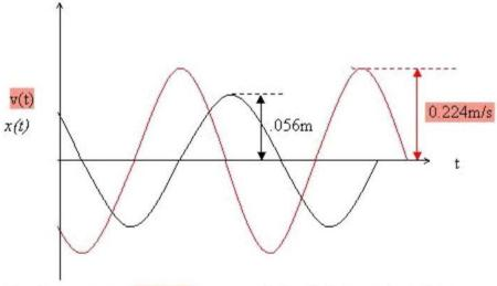
Displacement and velocity in example 1 with the initial condition x(0)=0.05 and v(0)=-0.1m/s.
