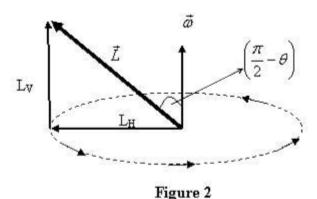
As the rod rotates  $L_V$  remains unchanged but  $L_H$  sweeps a circle with angular frequency  $\varpi$ . The rate of change of  $\vec{L}$  is therefore the same as that of  $L_H$ . The magnitude of the latter is  $\omega L_H$ . Since at the position shown, the tip of  $L_H$  is moving out of the paper, the direction of the change in  $L_H$  is also the same. This is the direction of principal axis 3. It thus follows that
