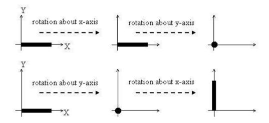
Different order of rotation about x and y axes leaves the rod being rotated with two different final orientations. In the upper set of rotations, first rotation of 90° is performed about the x-axis and is followed by a rotation of 90° about the y-axis. In the lower set, the order is interchanged.
