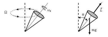
A precessing top (left) and its angular momentum and force mg acting on it (right).
