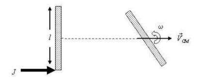
A rod being hit at one of its ends giving it an impulse J(left) and its position and orientation of the rod some time after the impact(right).
