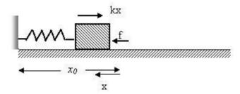
A spring-mass system with friction when the spring is compressed. Force applied by the spring and frictional force are both shown.
