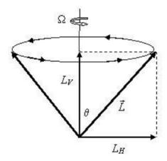
Angular momentum vector moving on the surface of a cone at a constant rate. Its vertical and horizontal components are Ly and LH, respectively.
