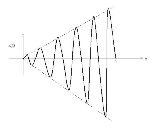
Forced oscillations of an undamped at resonance
