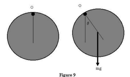
This is a case where a rigid body is moving under distributed forces so we use angular momentum to describe its motion. The equation of its motion therefore is
