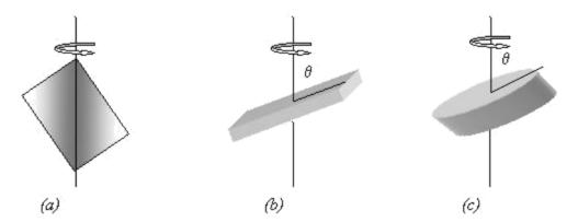
Find the rate of change of angular momentum of (a) a rectangular sheet rotating about its diagonal, (b) a rectangular sheet rotating about an axis passing through its centre, and (c) a thin disc rotating about an axis passing through its centre.
