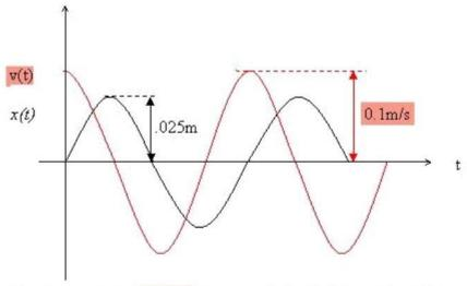
Displacement and velocity in example 1 with the initial condition x(0)=0 and y(0)=0.1m/s.
