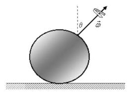
A spinning ball put on a rough floor with its angular velocity at an angle with the vertical.
