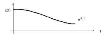
Displacement vs. time for a heavily damped oscillator
