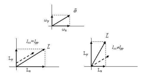
Direction of  $\vec{L}$  for a given  $\vec{\varpi}$  (upper figure). If  $I_{xx} = I_{yy}$ ,  $\vec{L}$  and  $\vec{\varpi}$ , shown by dashed arrow, are parallel (lower left). If  $I_{xx} \neq I_{yy}$ ,  $\vec{L}$  and  $\vec{\varpi}$  are not parallel (lower right).
