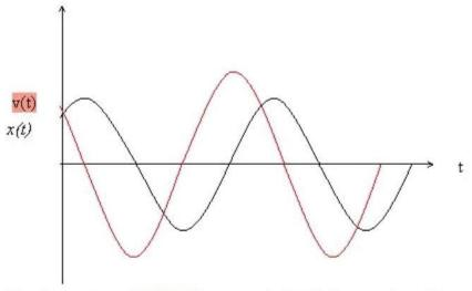
Displacement and velocity in example 1 with the initial condition x(0)=0.05 and v(0)=+0.1 m/s.
