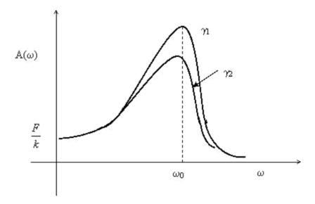
Amplitude as a function of frequency of applied force for two different values of  $\gamma$  with  $\gamma_1 < \gamma_2$ .
