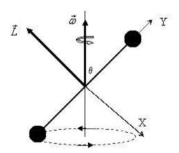
A thin massless rod with point mass m at both its ends rotating about a vertical axis. The principal axes are shown as X and Y axis with Z perpendicular to the XY plane.
