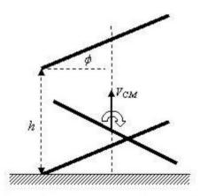
A rod dropped from a height rebounds from the floor and starts rotating. The CM moves only in vertical direction
