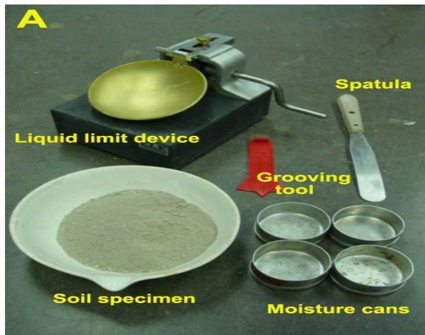
Fig: Shows Liquid limit test apparatus
