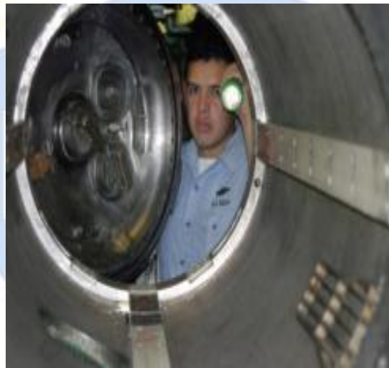
Fig: Visual inspection of a torpedo tube aboard a Navy attack submarine
