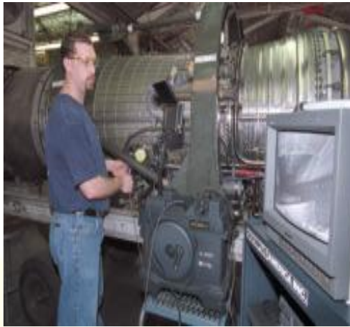
Fig: An inspector at Tinker Air Force base gets a magnified view of an engine's high-pressure turbine area with a new digital fiber-optic bore scope.
