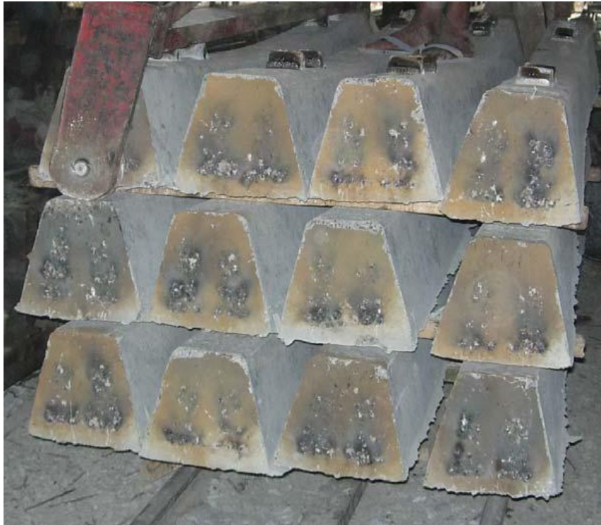
Figure: End of pre-tensioned railway sleepers
