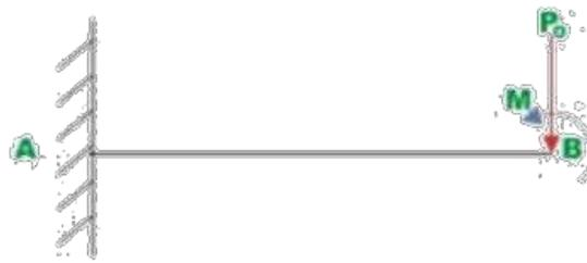
**Fig.23.3(a) Cantilever beam**
