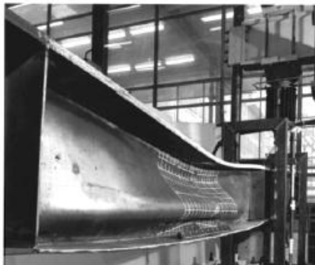
Figure 2. Vertical web buckling.
