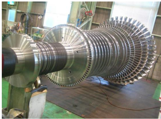
Figure: Steam Turbines
