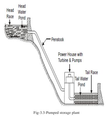
Fig-3.3-Pumped storage plant
