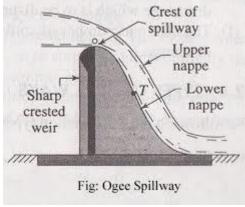
Fig-3.6- over flow spillway
