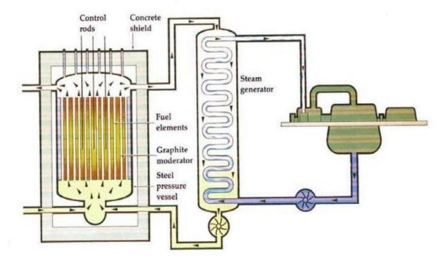
Fig-4.6- Gas cooled reactor
