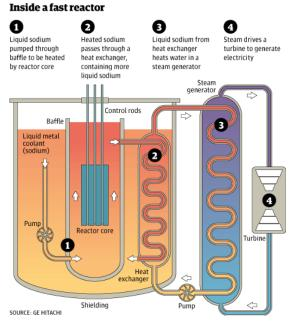
Fig-4.5-Fast breeder reactor
