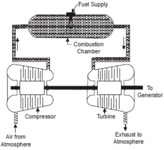
Fig-2.10-Open Cycle Gas Turbine
