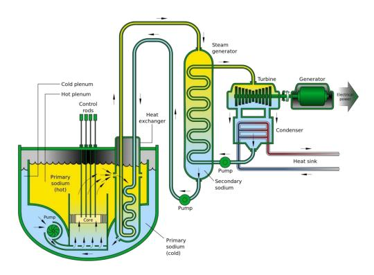
FIG.4.4-Sodium Graphite reactor
