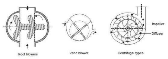
The blowers are usually driven from the engine cranks shaft by mean of Spur, helical or herringbone gears, silent chains or V-belts at a speed 2-3 times the engine speed. In the case of turbo-supercharger, the super charger is coupled to a gas turbine in which the exhaust of the engine is expanded.
