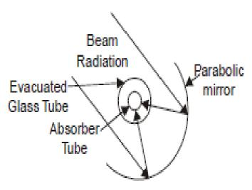
Fig-3.8- Solar collector
