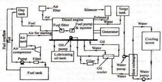
Fig-2.2-Layout of diesel plant
