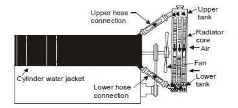
Fig-2.8-Natural Circulation Cooling System
