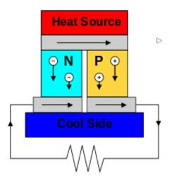
Fig-2.14- thermo electric system
