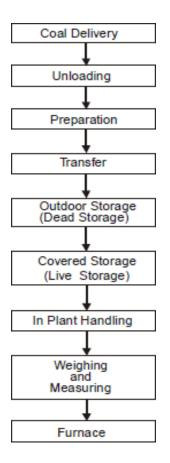
Fig-1.3-steps in coal handling
