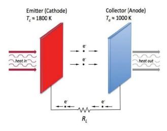
Fig-2.15- Thermo Ionic Convertor
