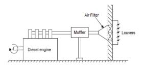
Fig-2.7-Air Intake System
