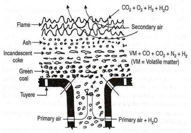
Fig-1.16- Underfeed Principle
