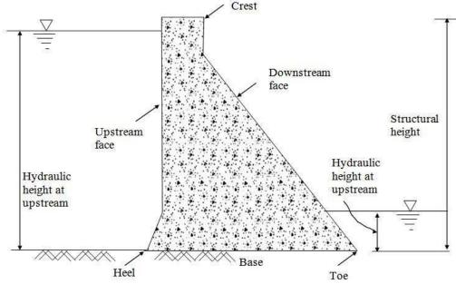
Fig-3.4- Gravity dam
