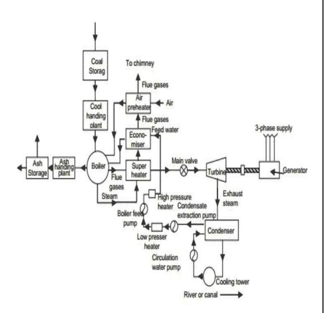
Fig-1.1- layout of steam power plant
