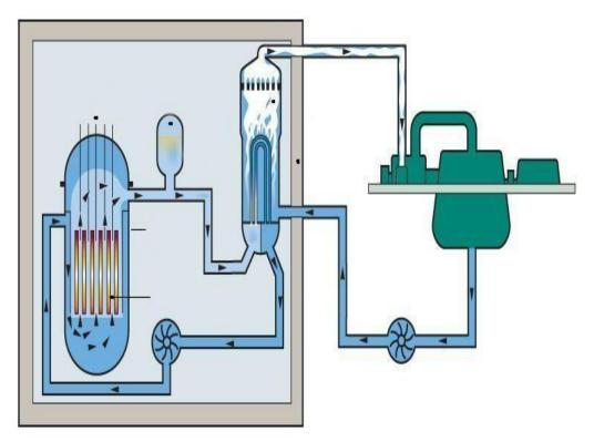
Fig-4.2- pressurized water reactor
