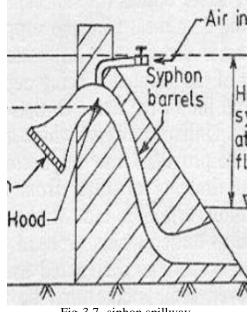
Fig-3.7- siphon spillway
