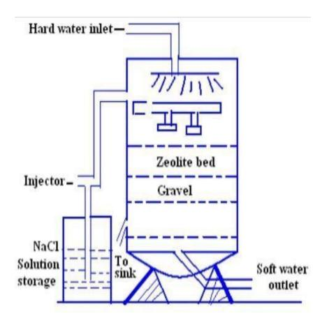
Fig-1.35- Zeolite Process
