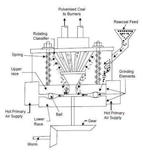
Fig-1.23-Ball and Race Mill
