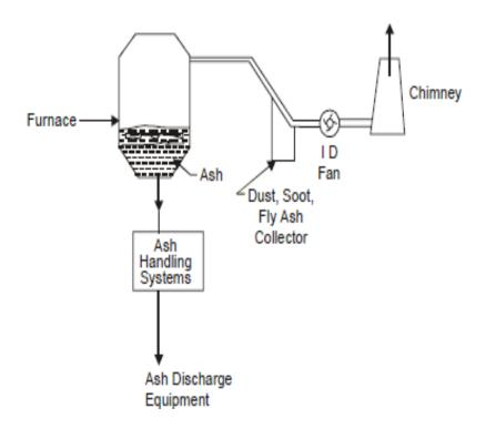
Fig-1.11-Ash handling system
