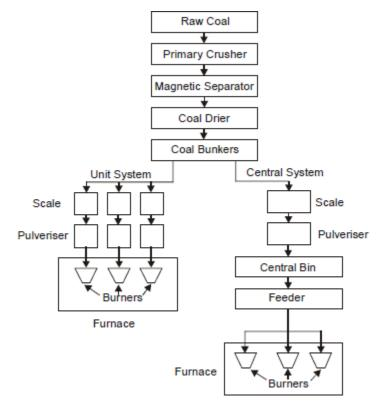
Fig-1.21- Components of pulversied fuel burning
