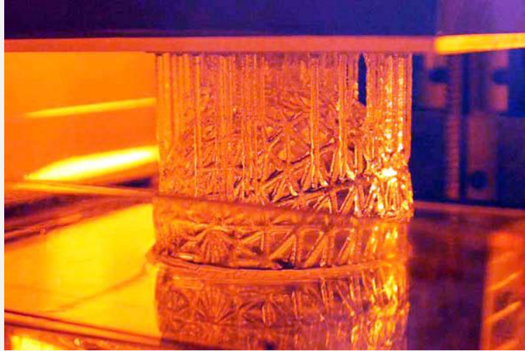
SLA printers often use an orange filter to screen out unwanted UV light.
