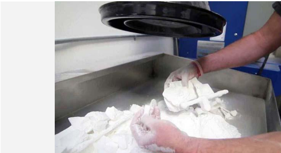
Excess powder being cleared away after SLS printing.
