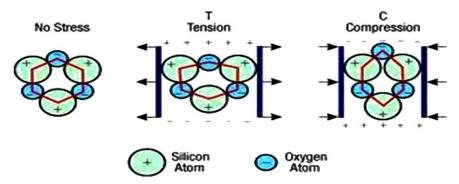
Fig. Piezo electric effect in quartz crystal
