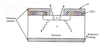
Fig. Construction of typical LED
