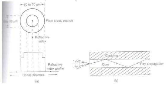
Fig (i). Single mode step index fiber; (a) Cross sectional view and refractive index profile; (b) Ray propagation
