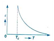
Fig. Variation of dielectric constant with temperature
