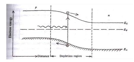
Fig. The generation & subsequent separation of an electron – hole pair by photon absorption within the depletion region of a p - n junction
