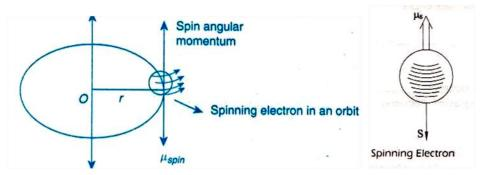
Fig. Spin magnetic moment of electrons
