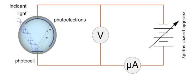
Figure Black diagram of Photo electric effect
