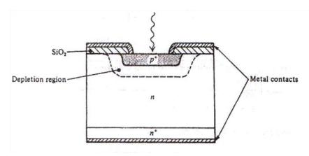
Fig. Typical silicon photo diode structure for photoconductive operation
