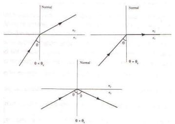
Fig. Total internal reflection.
