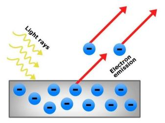
Figure Photoelectric effect
