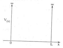
Fig.4.4 Square potential well infinite height
