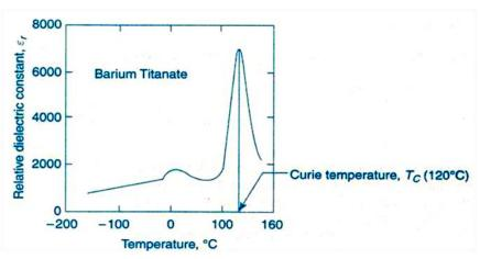
Fig. Variation of dielectric constant with temperature
