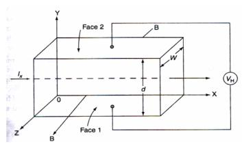
A semiconductor applied to current and magnetic field perpendicularly in Hall Effect
