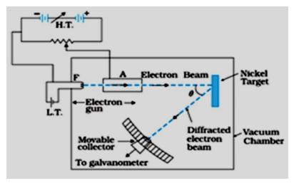
Figure 6Davisson and Germer's experimental arrangement for verification of matter waves
