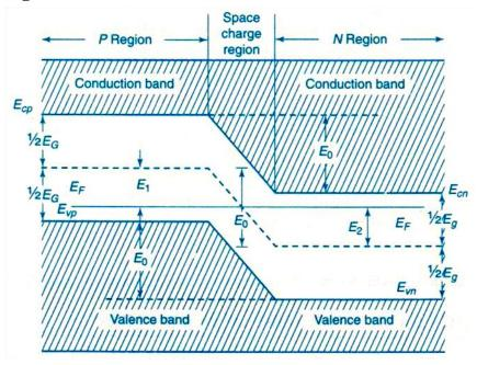
Fig. Energy level diagram of PN junction diode
