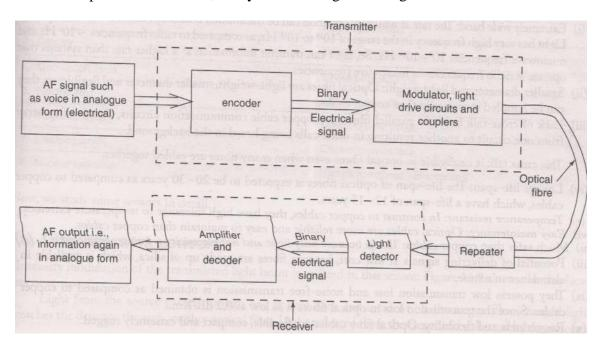
Fig. Block diagram represents optical fibre communication system
