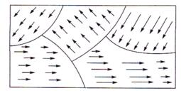
Fig. : Different possible orientations of domains
