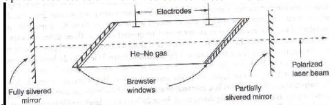
Fig. Helium-Neon gas laser
