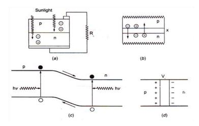
Fig. (a) p-n junction solar cell with load resistance,  $R_L$  (b) Diffusion of electrons & Holes (c) Energy band diagram of solar cell (d) Formation of the open circuit voltage  $V_o$
