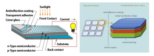
Fig. A typical solar cell consists of a glass or plastic cover, an antireflective coating, a front contact to allow electrons to enter a circuit, a back contact to allow them to complete the circuit, and the semiconductor layers where the electrons begin and complete their journey.
