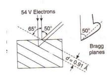
Figure 8 Bragg planes in Nickel crystal
