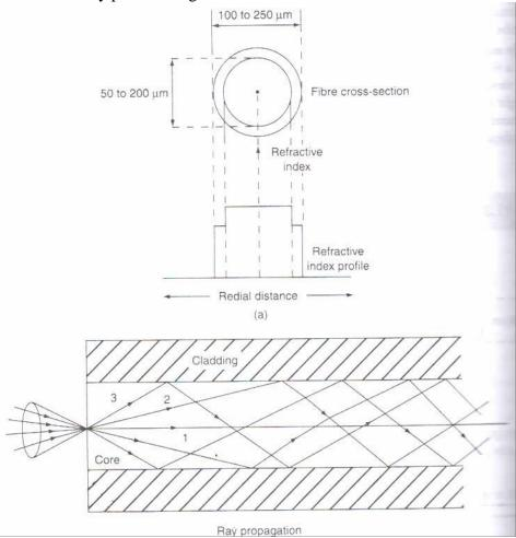
Fig. (ii).Multimode step index fibre(a)Cross sectional view and refractive index profle(b)Ray propagation
