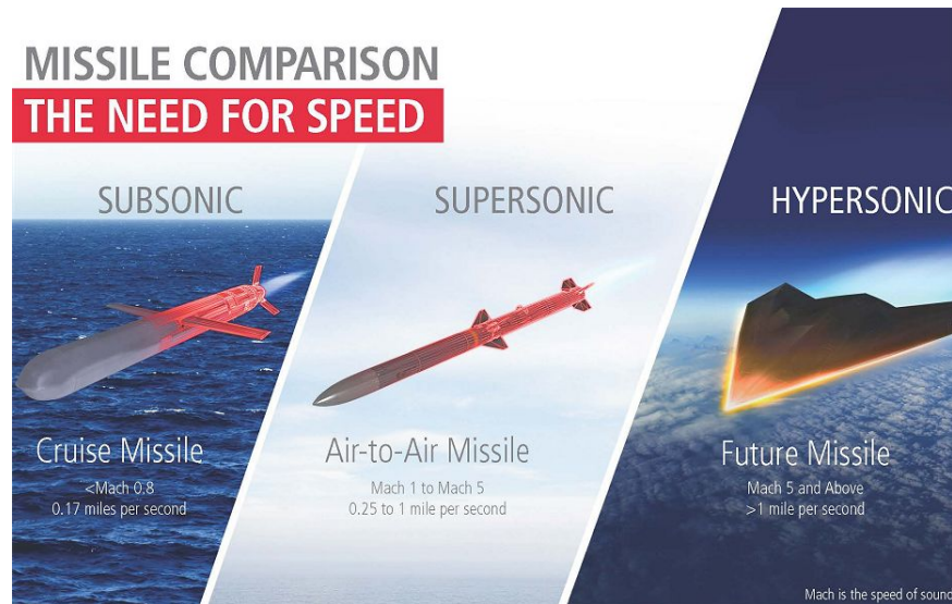
FIGURE 1.6: Missiles on the basis of its type
